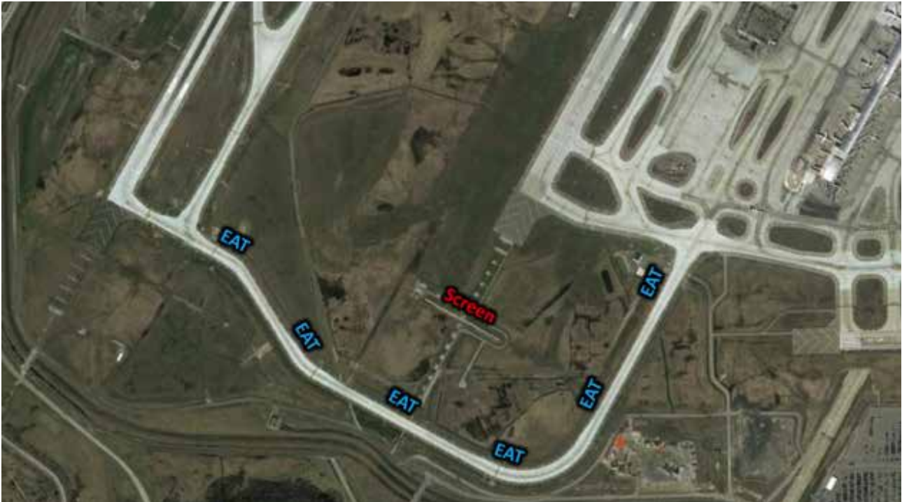
Fig 5: End Around Taxiway by-passing Threshold 04R at Detroit-Wayne Intl. Airport (DTW)
