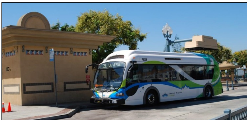
Figure 6. BEB charging station at the PTC
