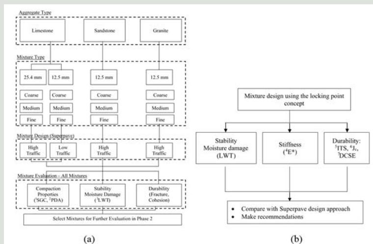
1 SGC: Superpave Gyrotory Compactor; 2 PDA: Pressure Distribution Analyzer; 3 LWT: Hamburg Loaded Wheel Tracking; 4 E\*: Dynamic Modulus; 5 ITS: Indirect Tensile Strength; 6 Jc: Critical J-integral; 7 DCSE: Dynamic Creep Strain Energy
