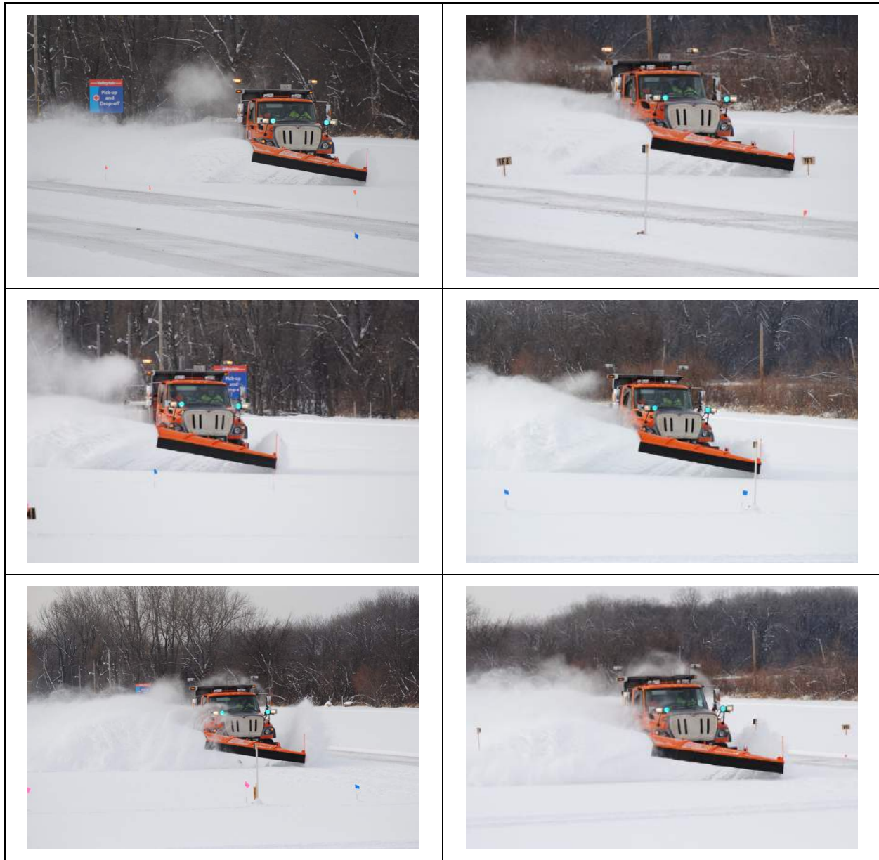
Figure 11. Evaluation of replication: two photos each of three lanes plowed at the same speed. Lanes shown are Valley Fair 1 (top), 2 (middle) and 3 (bottom), all plowed at 30 mph.
