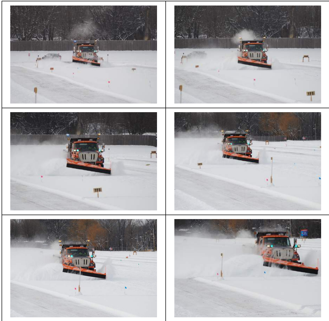
Figure 7. Valley Fair Lane 7, truck speed 25 mph, December 12, 2016; very dry fine snow with uniform structure, approximately 5 inches thick. Photos at approximately 100-foot increments through the zone of constant speed.
