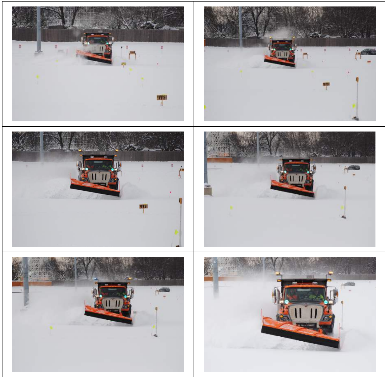
Figure 9. Valley Fair Lane 9, truck speed 25 mph, December 12, 2016; very dry fine snow with uniform structure, approximately 5 inches thick. Photos at approximately 100-foot increments through the zone of constant speed.
