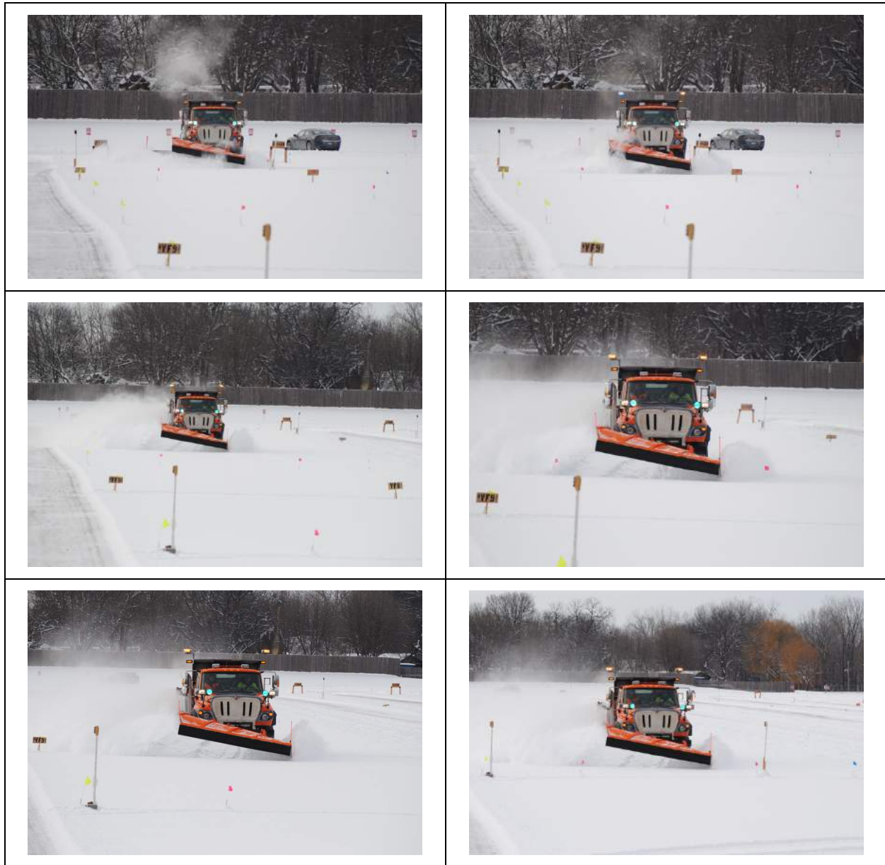
Figure 8. Valley Fair Lane 8, truck speed 25 mph, December 12, 2016; very dry fine snow with uniform structure, approximately 5 inches thick. Photos at approximately 100-foot increments through the zone of constant speed.
