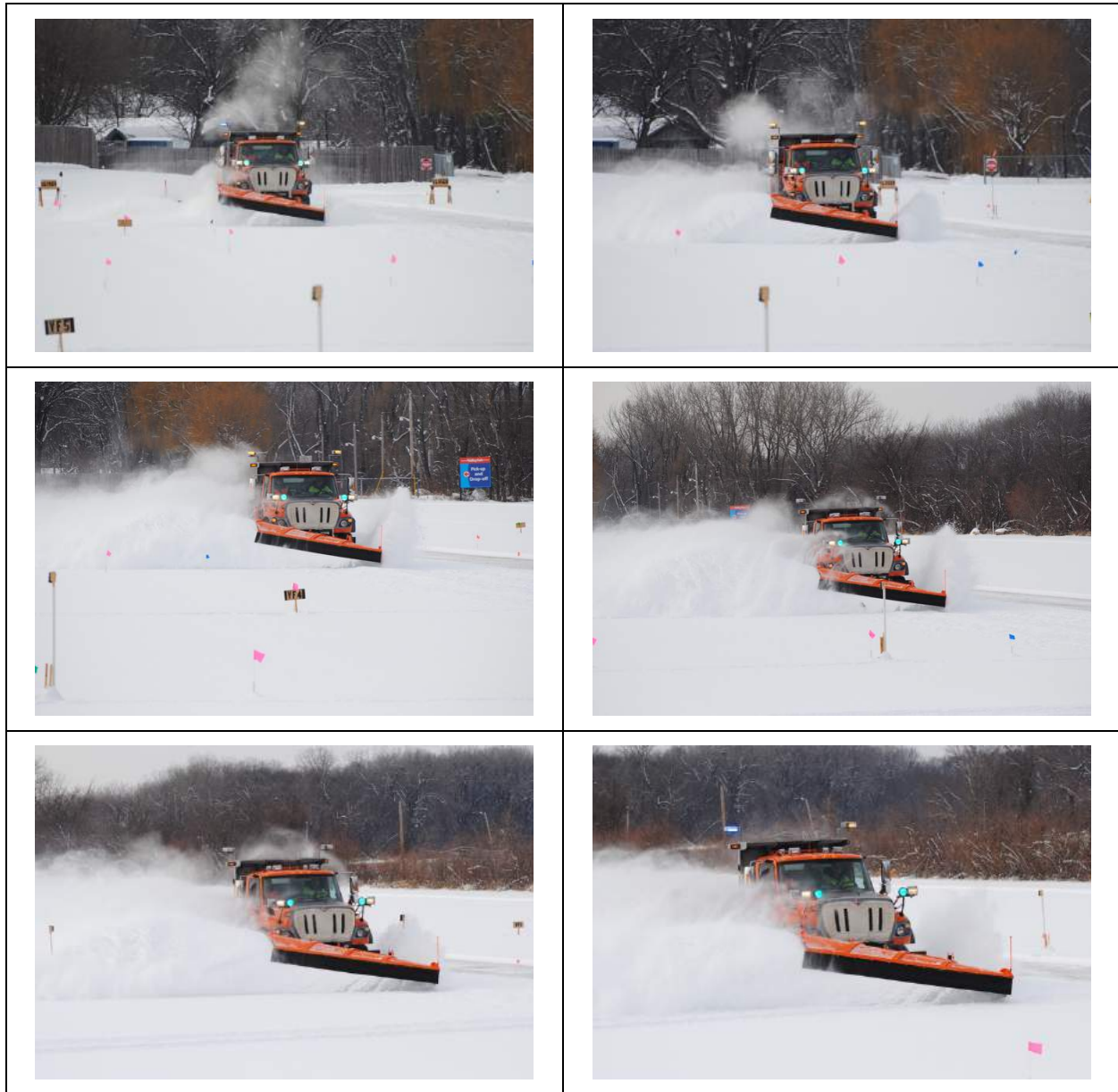
Figure 3. Valley Fair Lane 3, truck speed 30 mph, December 12, 2016; very dry fine snow with uniform structure, approximately 5 inches thick. Photos at approximately 100-foot increments through the zone of constant speed.
