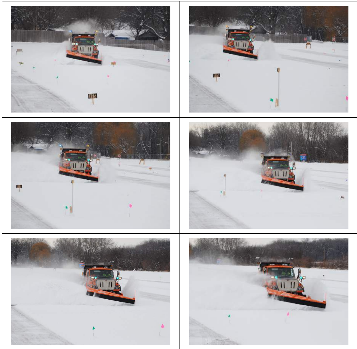
Figure 4. Valley Fair Lane 4, truck speed 35 mph, December 12, 2016; very dry fine snow with uniform structure, approximately 5 inches thick. Photos at approximately 100-foot increments through the zone of constant speed.
