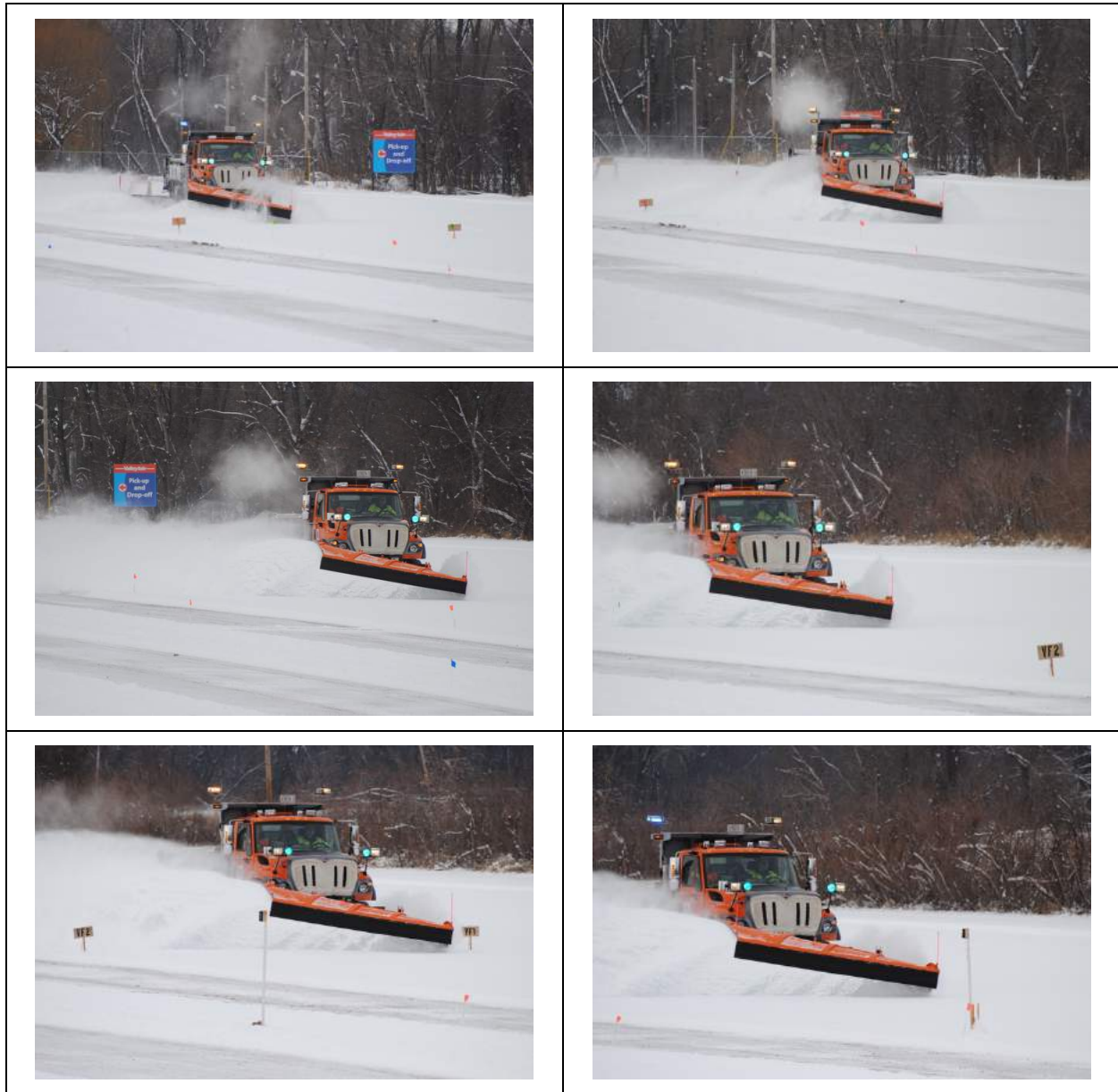
Figure 1. Valley Fair Lane 1, truck speed 30 mph, December 12, 2016; very dry fine snow with uniform structure, approximately 5 inches thick. Photos at approximately 100-foot increments through the zone of constant speed.
