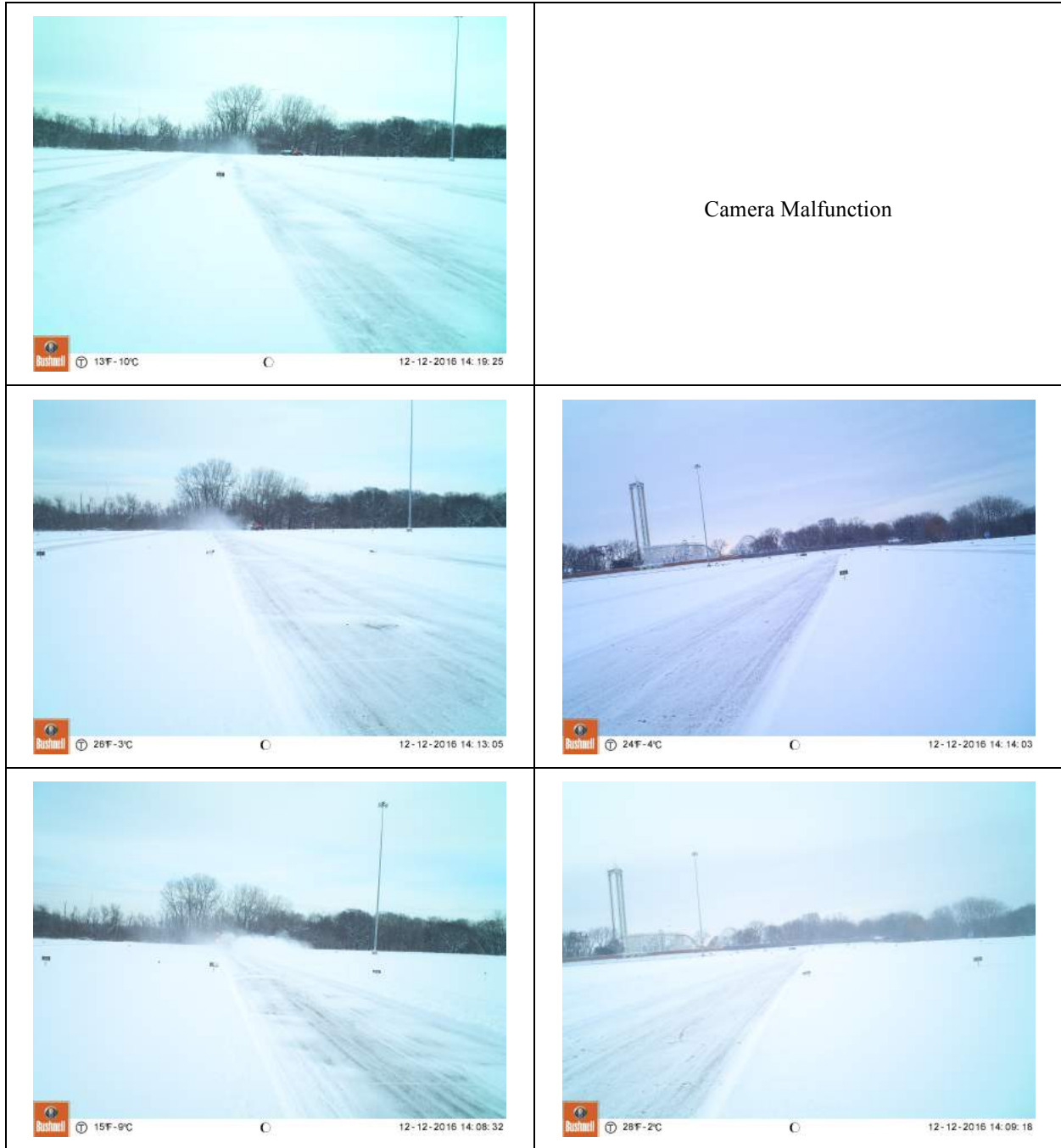
Figure 25. Evaluation of replication: two photos each of three lanes plowed at the same speed. Lanes shown are Valley Fair 4 (top), 5 (middle) and 6 (bottom), all plowed at 35 mph.
