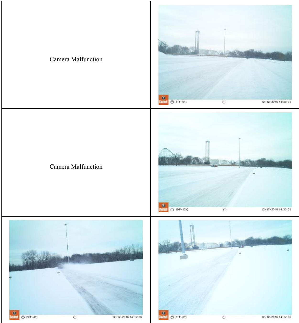
Figure 23. Evaluation of replication: two photos each of three lanes plowed at the same speed. Lanes shown are Valley Fair 7 (top), 8 (middle) and 9 (bottom), all plowed at 25 mph.
