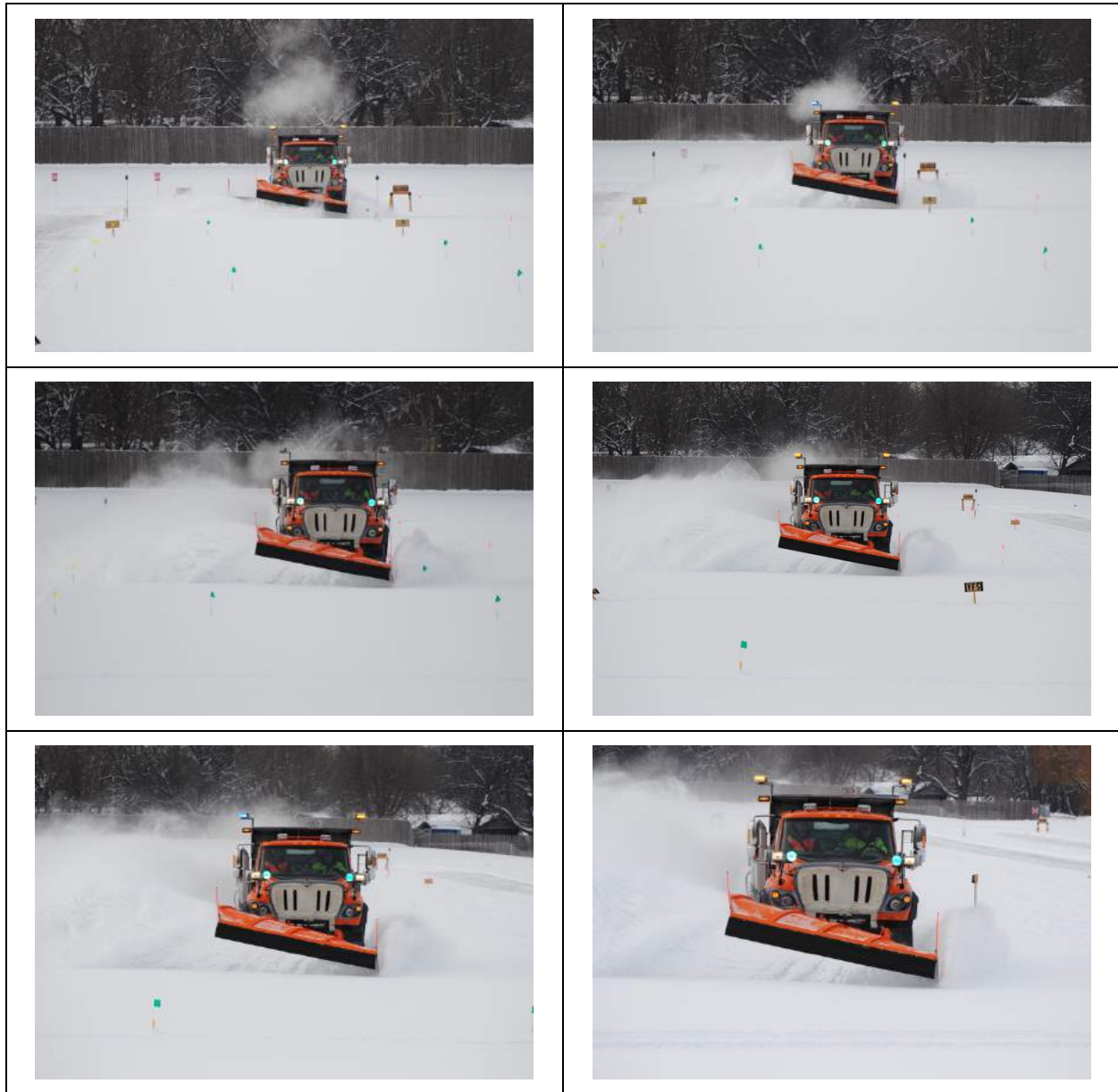
Figure 5. Valley Fair Lane 5, truck speed 35 mph, December 12, 2016; very dry fine snow with uniform structure, approximately 5 inches thick. Photos at approximately 100-foot increments through the zone of constant speed.
