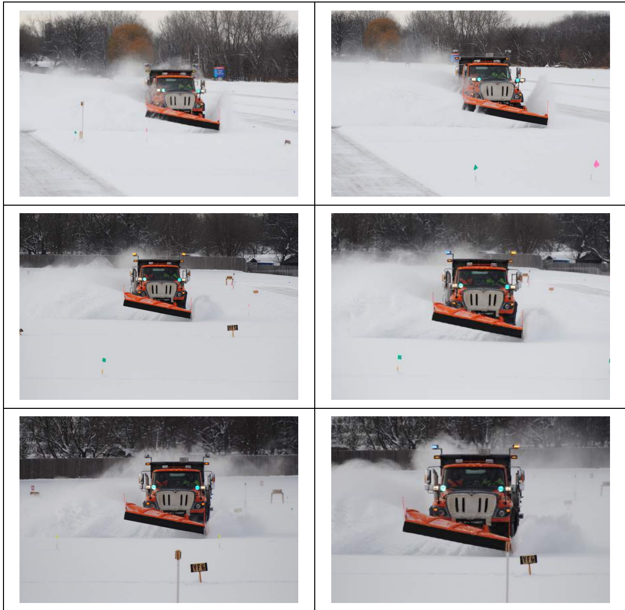
Figure 12. Evaluation of replication: two photos each of three lanes plowed at the same speed. Lanes shown are Valley Fair 4 (top), 5 (middle) and 6 (bottom), all plowed at 35 mph.
