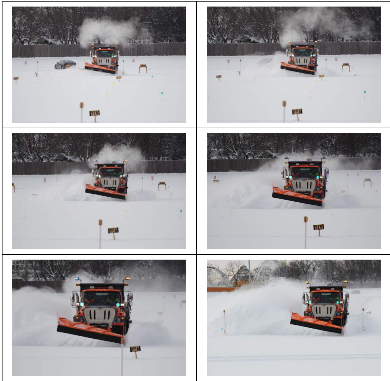
Figure 6. Valley Fair Lane 6, truck speed 35 mph, December 12, 2016; very dry fine snow with uniform structure, approximately 5 inches thick. Photos at approximately 100-foot increments through the zone of constant speed.
