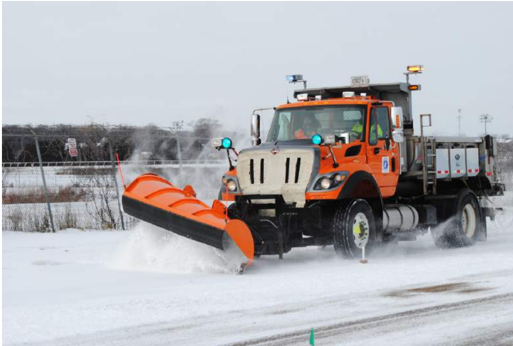
Figure 28 Typical MnDOT winter maintenance truck, circa 2016, outfitted with front, right wing and underbody plows, brine saddle tanks and rear deicer distribution system.
