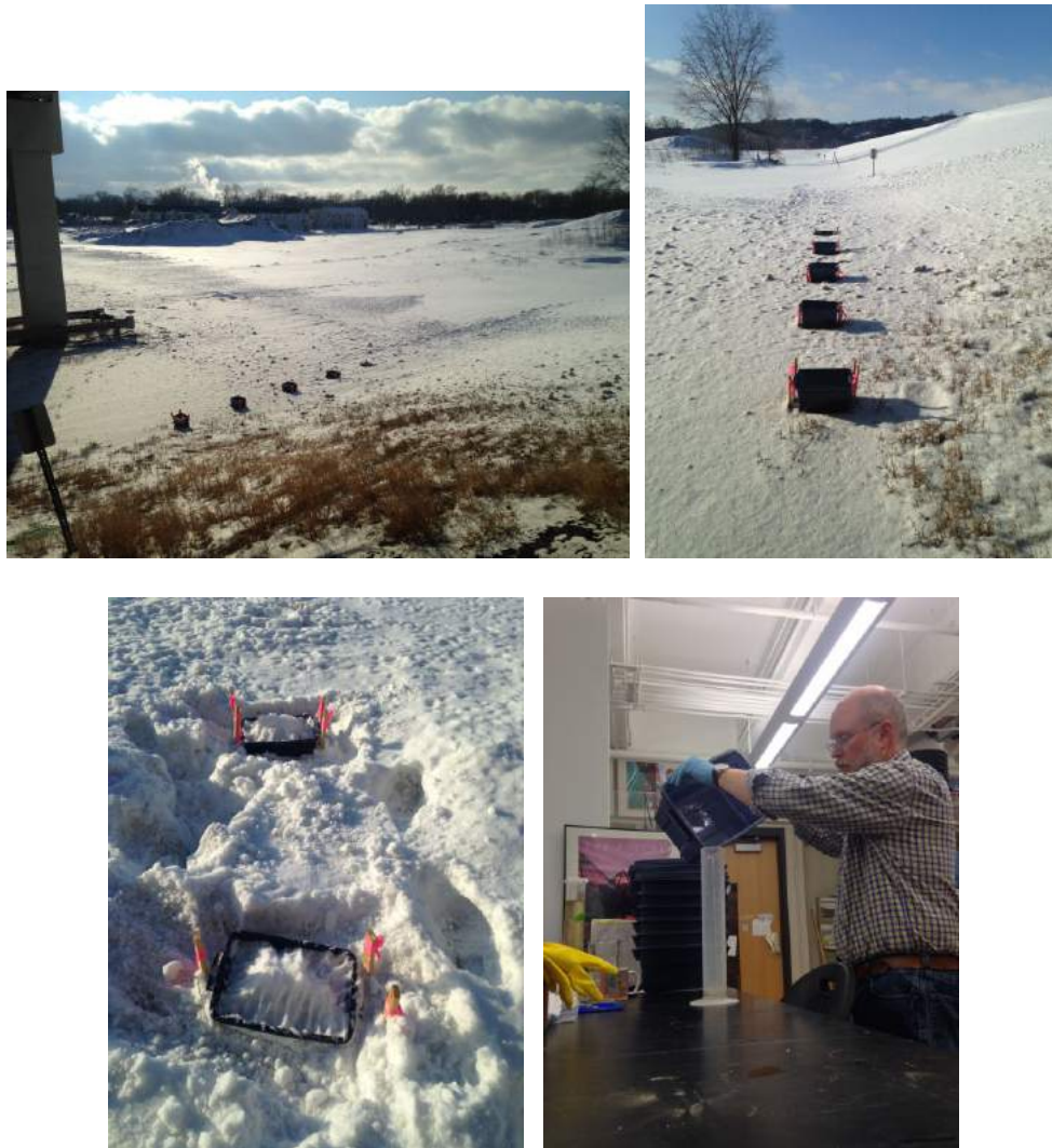
Figure 29 Plow cast experiment for the storm of February 3, 2016.
