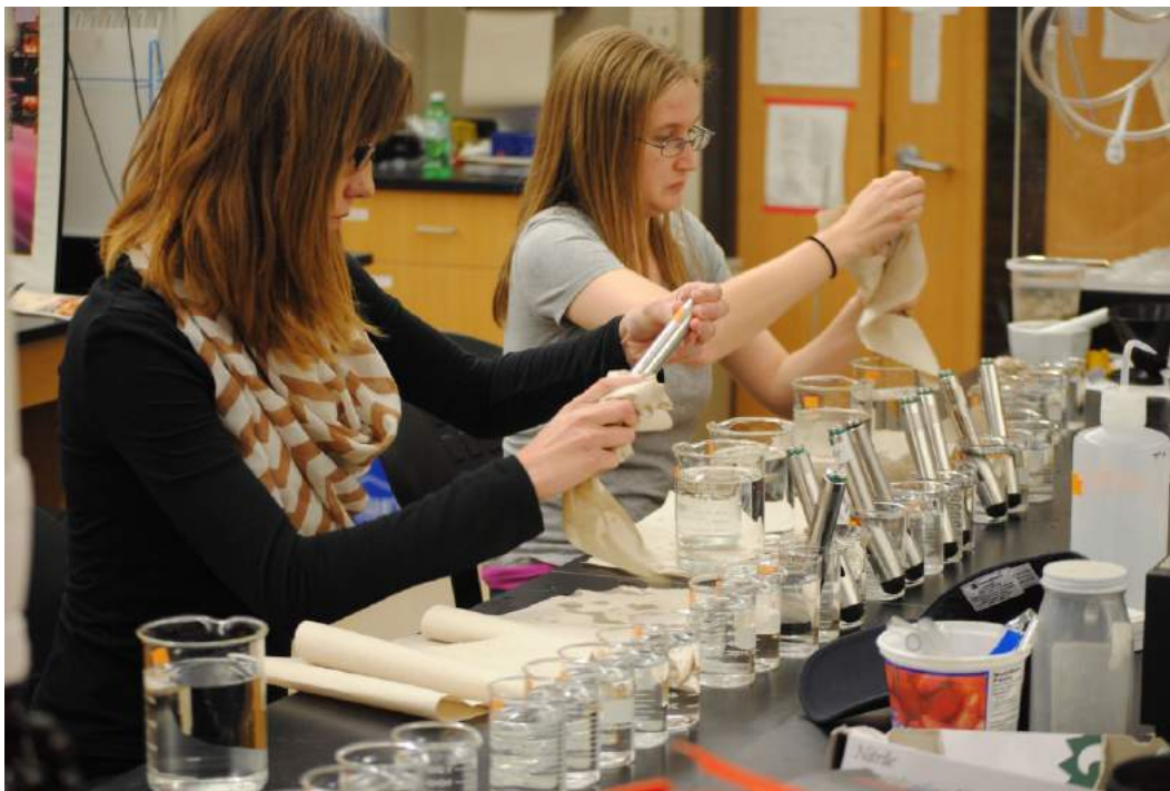
Figure 25 Calibration of conductivity measurement in ten total data loggers (Levelloggers). Solutions of various concentrations contained in beakers. Levelloggers being rinsed with deionized water and toweled dry between placement in solutions.
