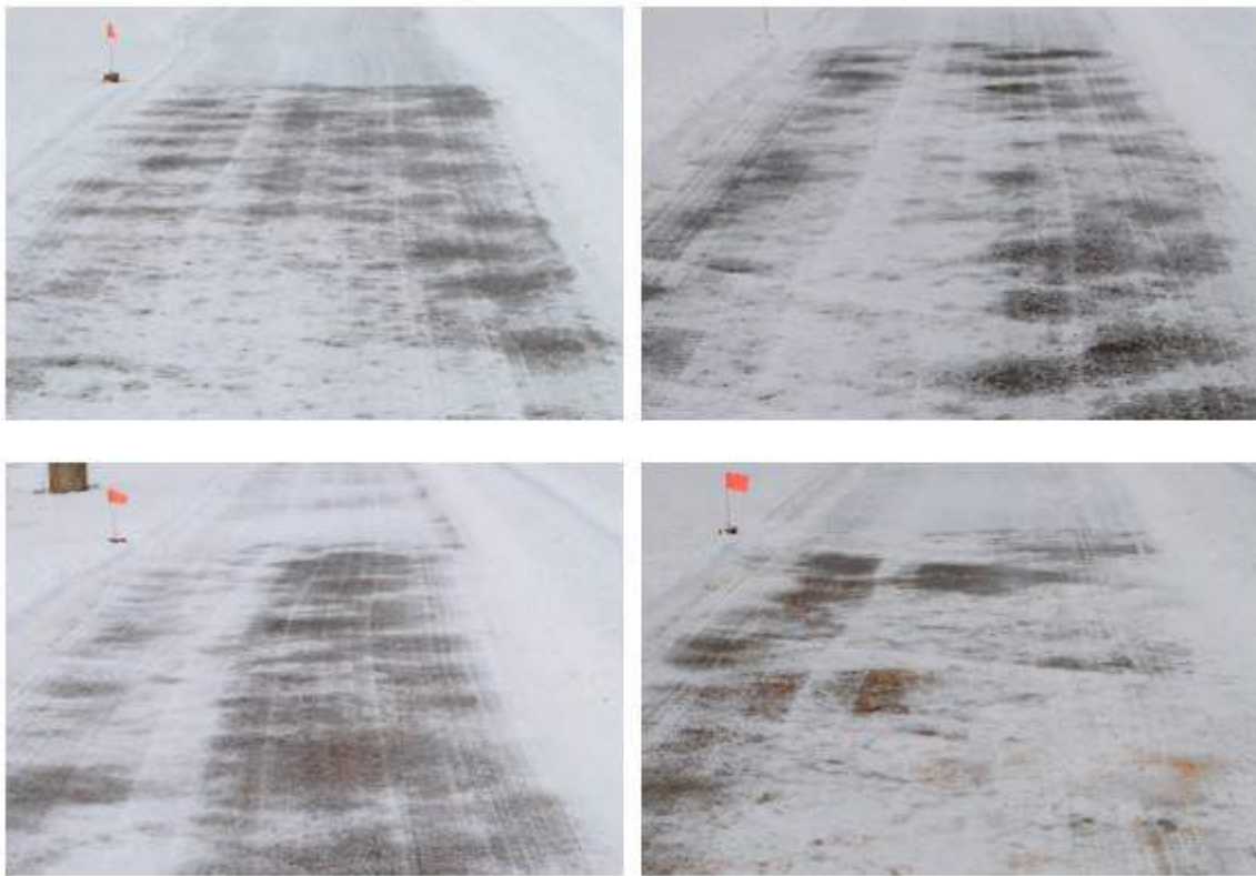
Figure 8 Pavements treated at 600 lbs/LM of different deicer solids with 15 gal/ton prewet of RG8 10% (90% salt brine) applied at the point of hand distribution: rock salt (top left), magnesium chloride (top right), calcium chloride (bottom left), and Ice Slice
