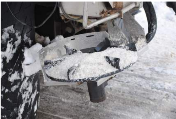
c) Salt distributor behind left rear wheel (not in motion/not being fed deicer at time of photo).
