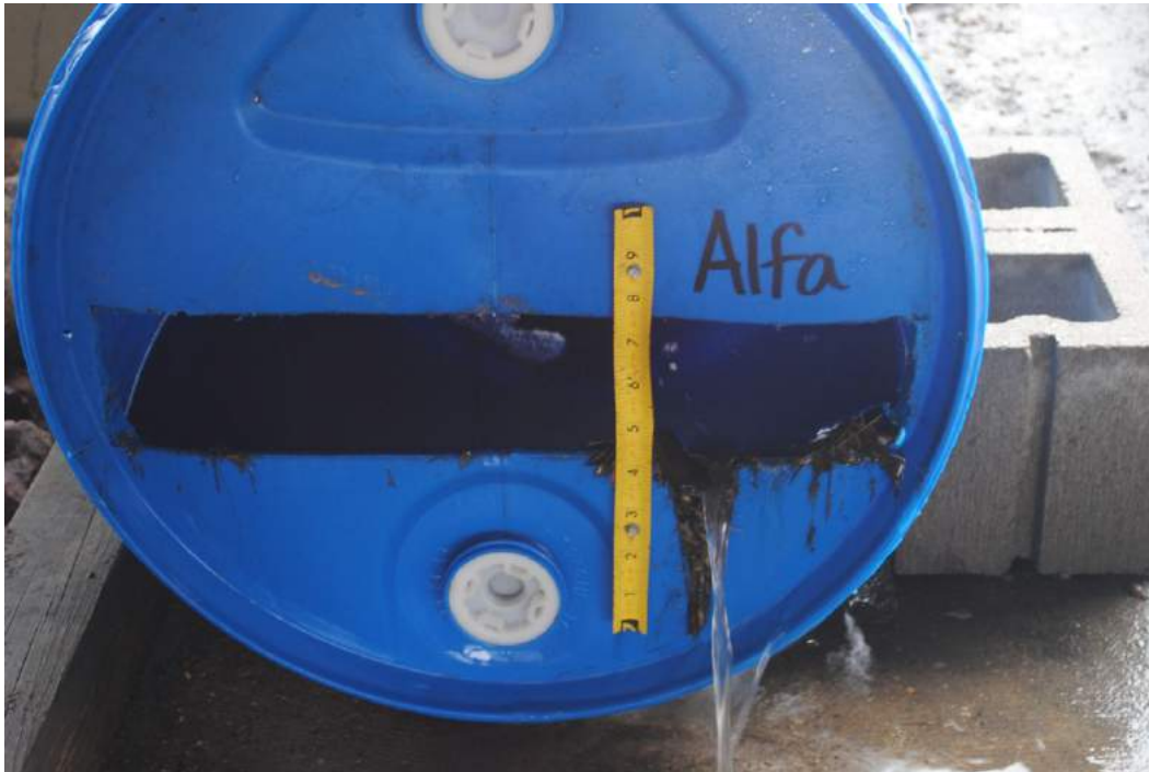
Figure 26 Debris clog at Location A, March 27, 2014.
