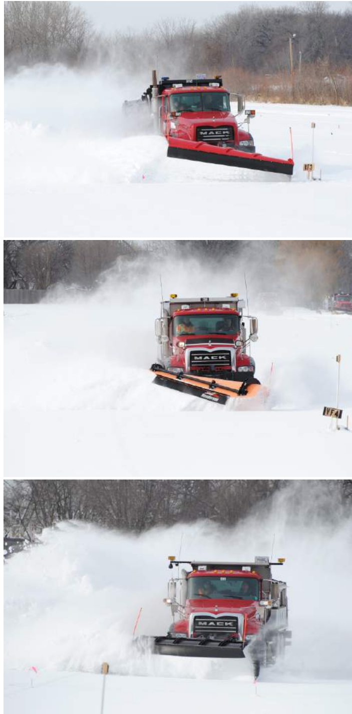
Figure 14 Comparison of one-way (top; VF3), poly (flex, center; VF4), and dozer (bottom; VF5) plows.
