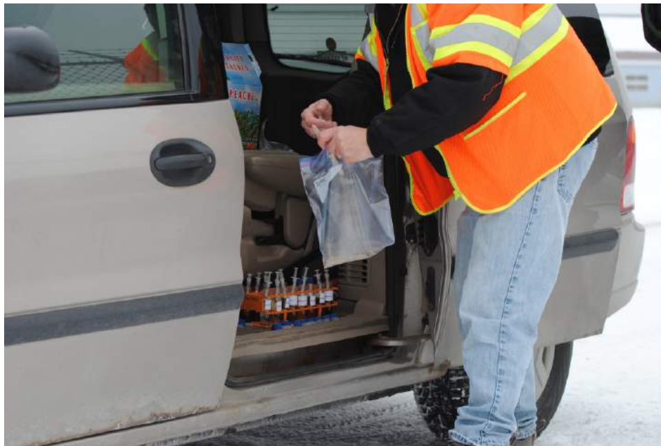
Figure 7 Application of prewet to premeasured amount of deicer: full lane width treatment using a 500 mL bottle as container of premeasured prewet (top); and compacted wheel track treatment using a 3 mL disposable syringe to field-measured the amount of prewet
