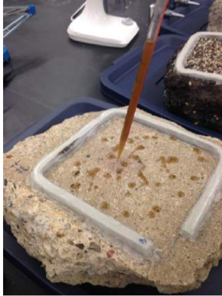
Figure 31 Anti-icer application to defined pavement area.
