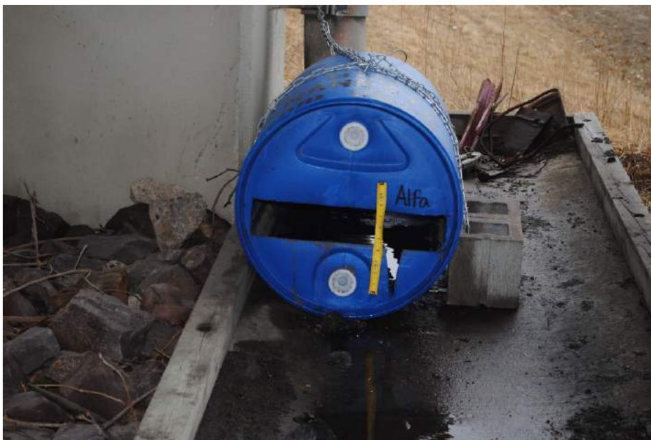
a) End view showing plastic drum with V-notch weir, broad weir, manual measurement tape, leveling chain/concrete masonry unit, and security chain.
