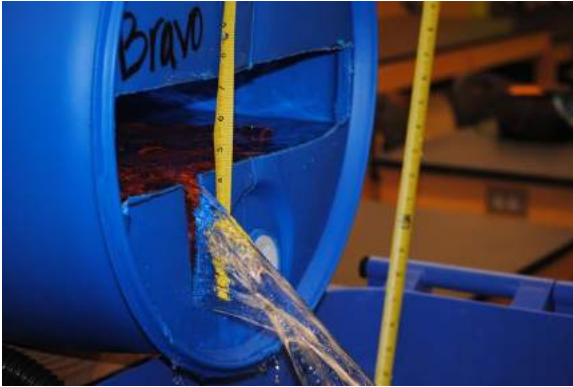
a) Flow through V-notch weir into receiving sump.
