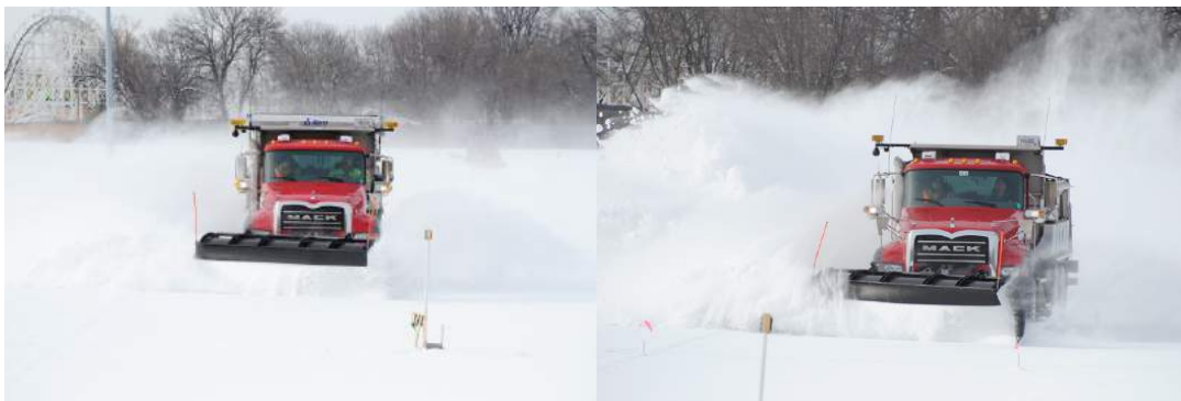
Figure 16 Comparison of dozer plows with differing cast and cloud characteristics: low, tight cast with little clouding (left; VF8); and broad, turbulent cast with widespread, thick clouding (right; VF5).
