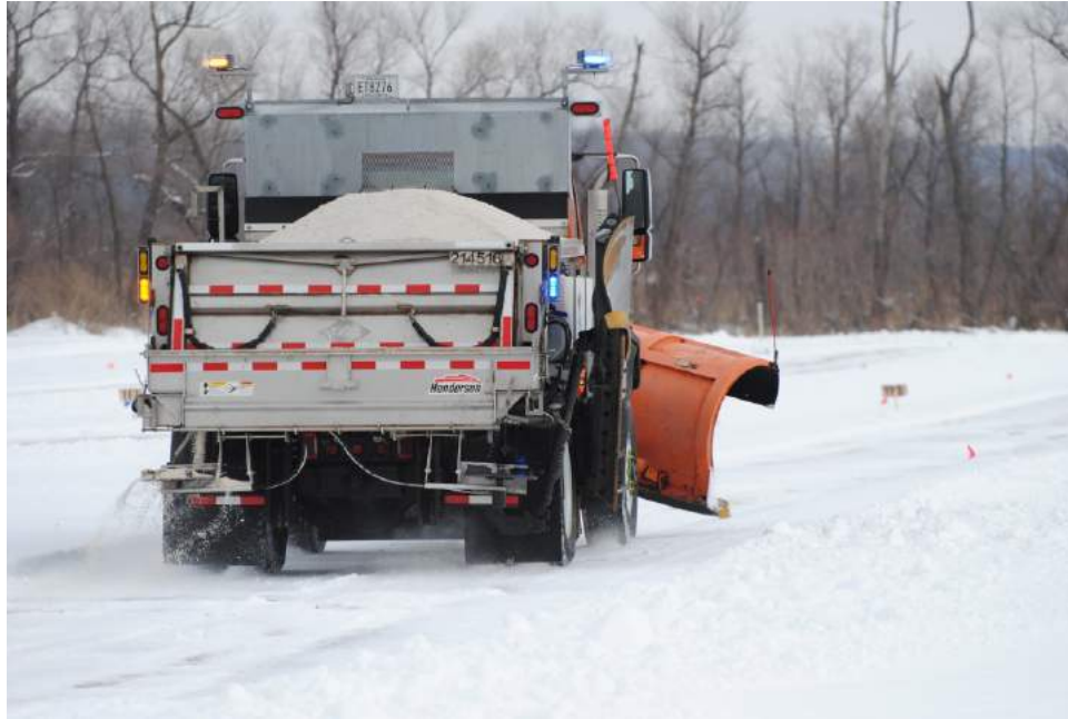
Figure 5 MnDOT truck spreading deicer off left rear while moving forward on a lane where plowing was done previously by another truck.
