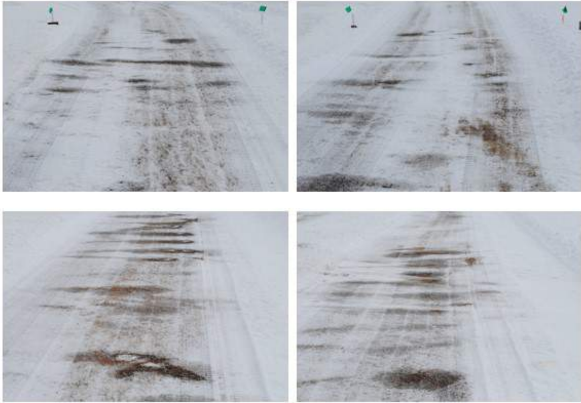
Figure 9 Pavements treated at 600 lbs/LM of different deicer solids with no prewet: rock salt (top left), magnesium chloride (top right), calcium chloride (bottom left), and Ice Slicer (bottom right). No traffic application. Photographs taken approximately 60
