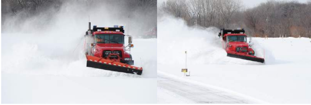
Figure 15 Comparison of one-way plows with differing cast and cloud characteristics: low, tight cast with moderate clouding (left; VF7); and broad, moderately high cast with thick, opaque clouding (right; VF6).
