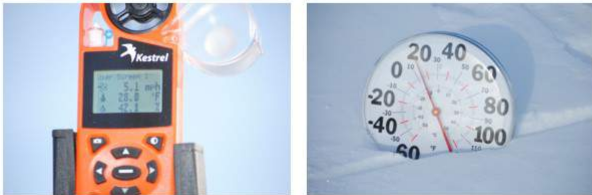
Figure 2 Weather monitoring tools: handheld weather station; dial thermometer.
