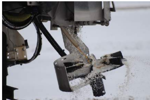
d) Prewet flow and deicer drop onto salt distributor (in motion at time of photo).
