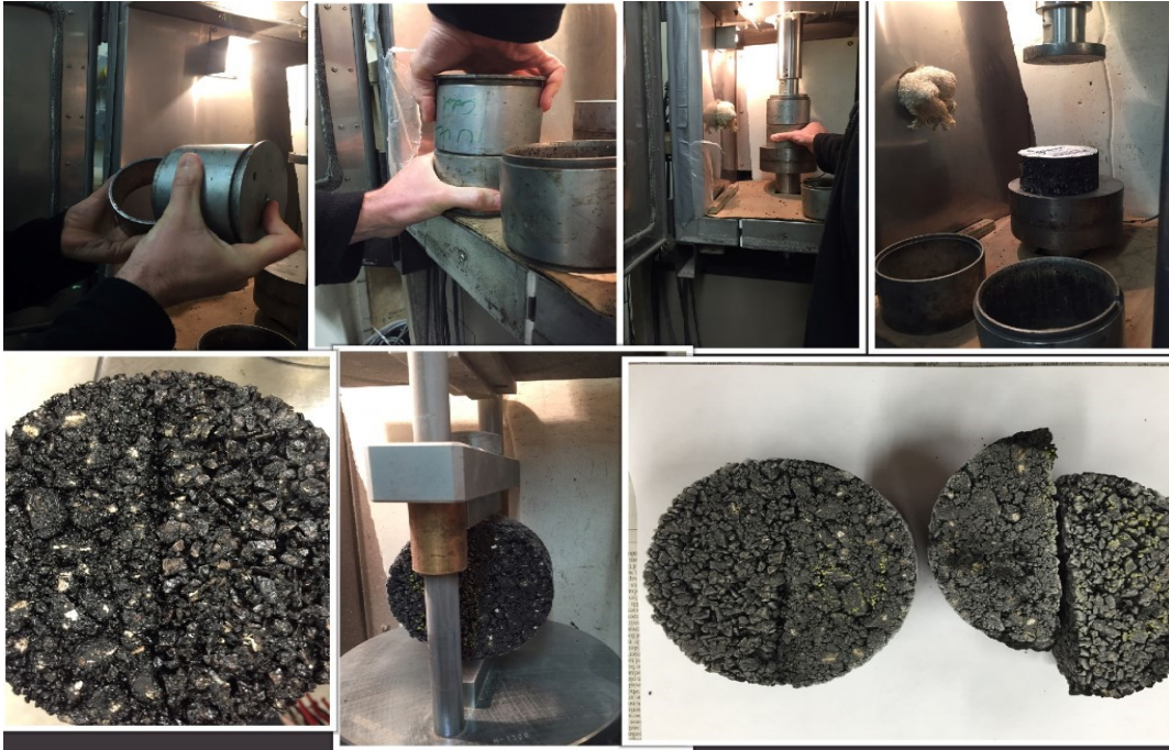
Figure 4.12: Additional photos of sample preparation and testing with half HMA and half patching material.
