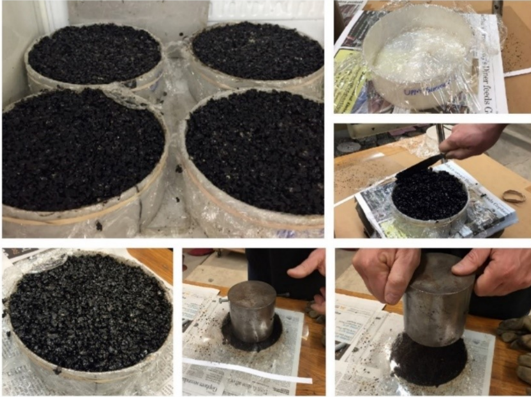
Figure 4.5: Sample preparation using plastic mold and manual compaction.
