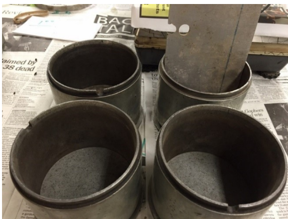
Figure 4.8: Sample preparation using steel mold and MTS compaction.
