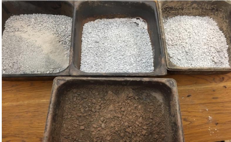
Figure 4.2: Aggregate residue from patching materials. Upper Left: Perma-Patch. Upper Middle: Summer Mix_UPM. Upper Right: Winter Mix_UPM. Bottom: Winter Mix_St Paul.
