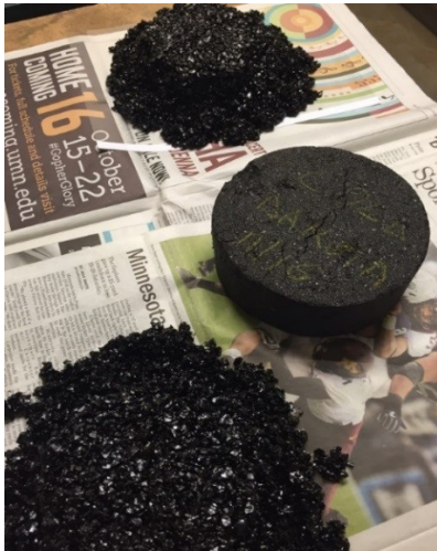
Figure 4.4: Sample preparation using gyratory compaction.
