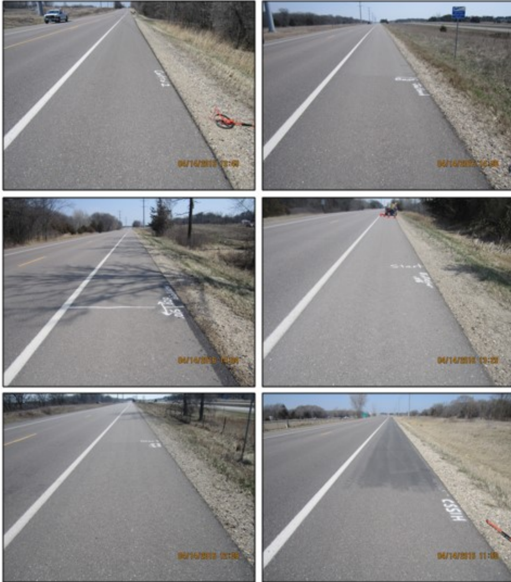
Figure 5.21 Year Two dry-condition photos clockwise from upper left: WB Control, Jointbond®, Biorestor® 0.015, CSS-1h, RePlay™, and Biorestor® 0.020.
