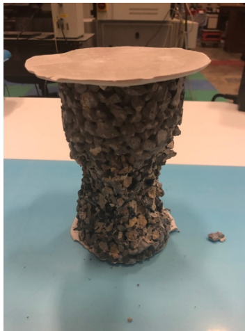
Figure 3.10 Typical pervious concrete specimen after unconfined compressive strength test
