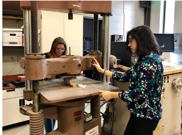
Figure 2.4 Split tensile testing
