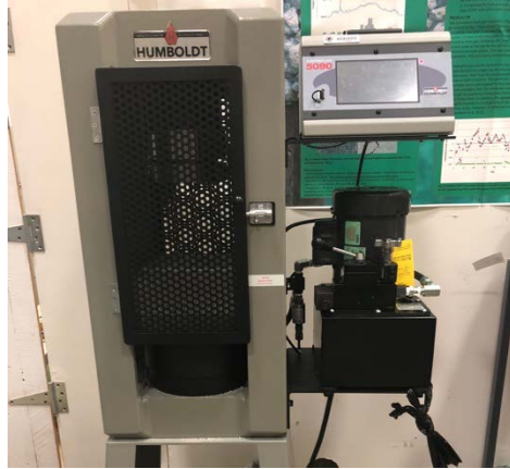
Figure 3.9 Unconfined compressive strength test machine (HCM-5090.3F): Phase IIb
