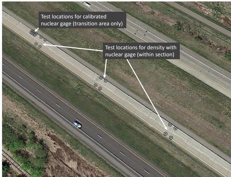
Figure 3.6 Typical layout for density calibration cores and nuclear density testing.
