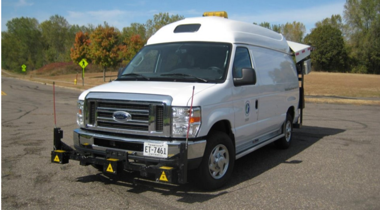
Figure 10.1 MnDOT digital inspection vehicle (DIV).
