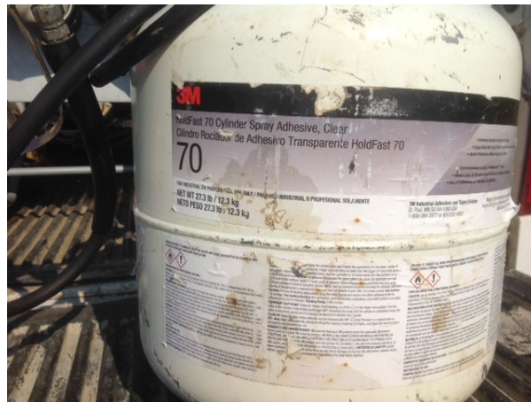
Figure 4.10 Adhesive used to secure non-woven geotextile fabric in Cells 705 and 805.
