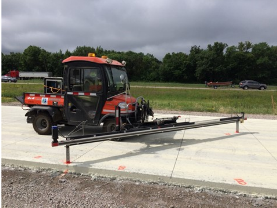
Figure 10.2 MnROAD ALPS2 device measures changes in concrete pavement surface shape due to warp and curl.
