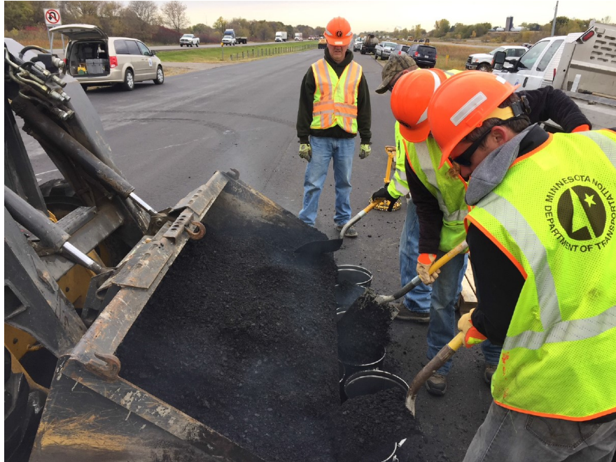
Figure 3.5 Transferring bulk samples to containers for distribution to NRRRA participants.
