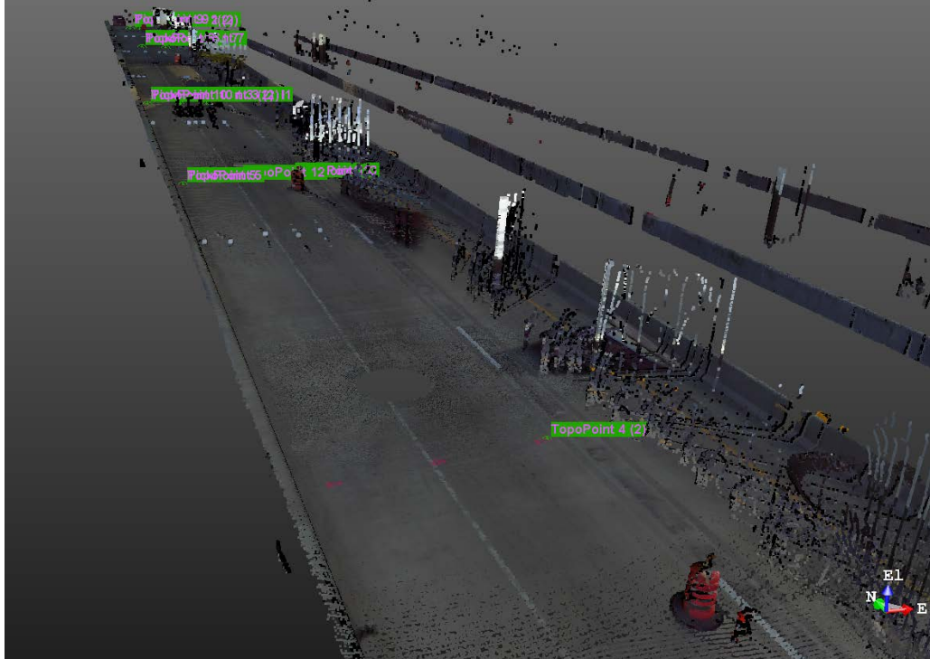
Figure 10. I-57 Bridge over Kankakee River – Laser scan compiled from cloud data.
