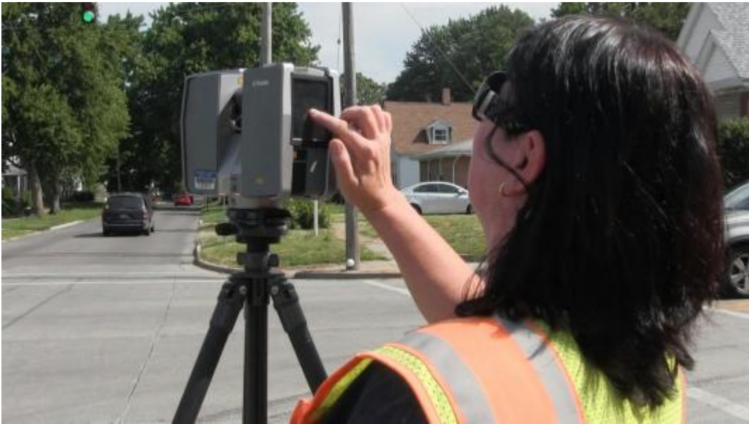
IDOT survey crew member surveying intersection with 3-D scanner out of the path of live traffic. Photo courtesy of IDOT.
