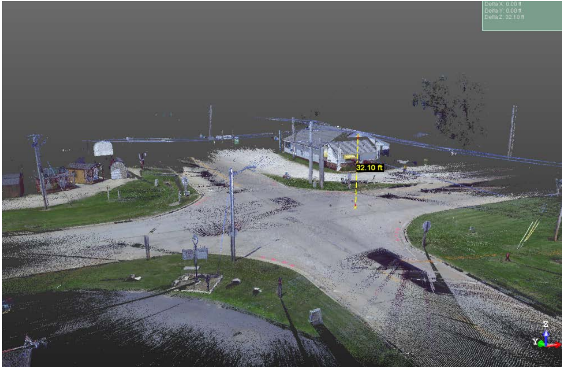
Figure 16. Route 178 and US 6 intersection, laser scanner generated point cloud with image superimposed. Scanning for utility wire heights for potential conflicts.
