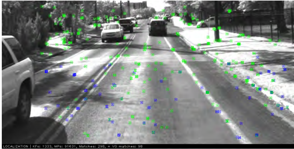
FIGURE 13. Localization in a prior map. Green keypoints represent matches from the prior map. Blue keypoints represent new detected features.
