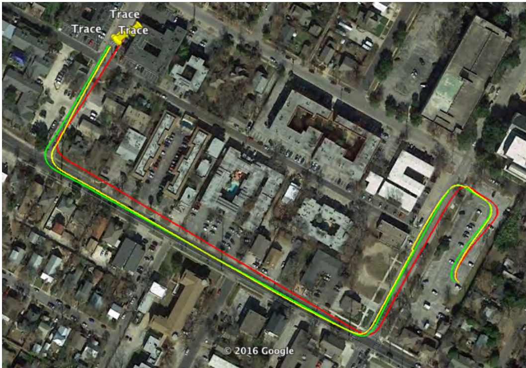
FIGURE 5. Google Earth visualization of the GNSS/INS (yellow), GNSS/INS-aided-SLAM (green), and SLAM-only (red) trajectories.
