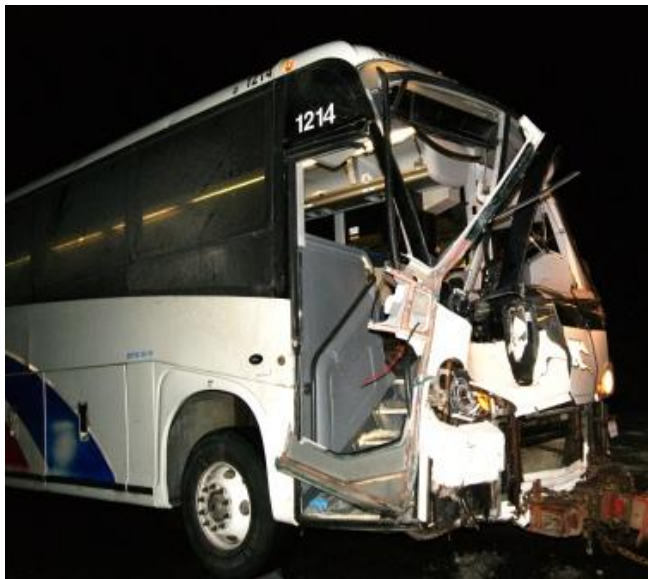
Figure 9 – Direct icefall impact damage to bus near Terrace, British Columbia, courtesy of Terrace Daily Online, February 5, 2011.
