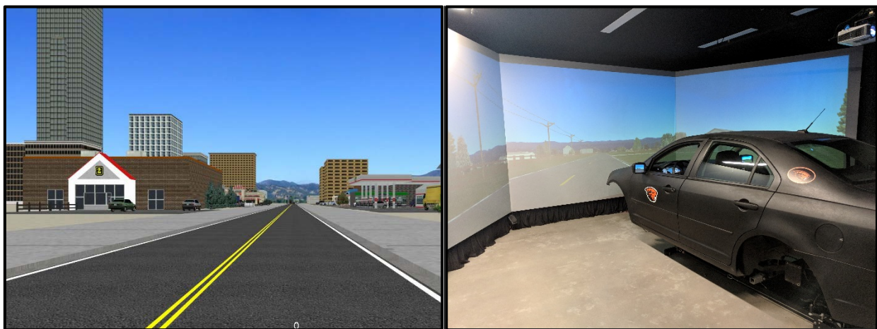
Figure 6.2: Simulated environment in OSU driving simulator, from the participant's perspective inside (left) and from outside (right) the vehicle
