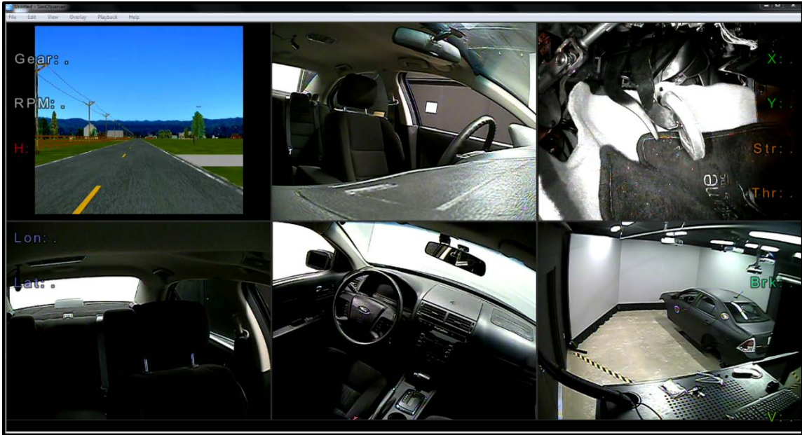
Figure 6.4: Screenshots of the six views from SimObserver. Clockwise from top left: simulated scene as projected on the screen; driver’s upper body and hands on steering wheel; acceleration and brake pedals in vehicle; entire simulator viewed from outside the vehicle; steering wheel and dashboard; and driver’s face.
