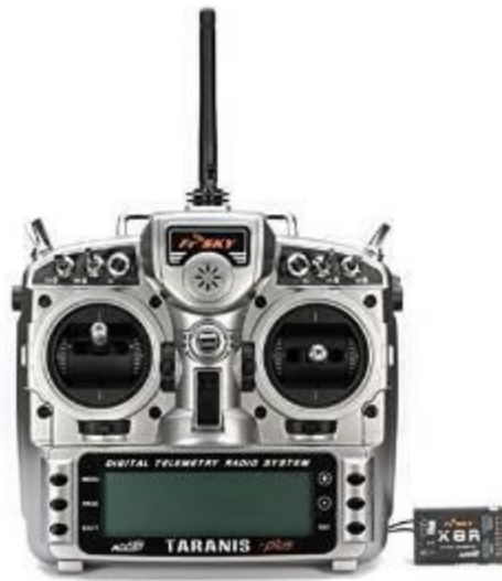
Figure 21. Example of an RC controller used in mobile environment (FrSky Taranis X9 X9D Plus RC Controller).
