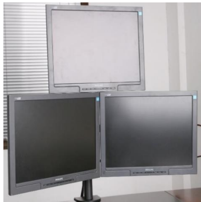
Figure 10. Example of pyramid display set up. Inverted pyramid setups are also used (Pyramid Display).
