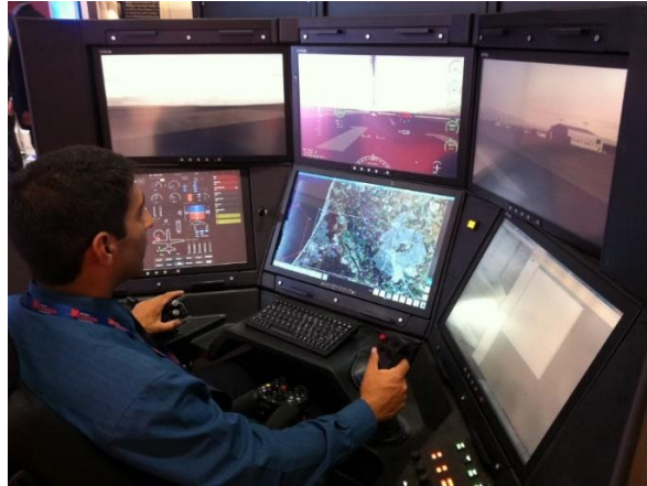
Figure 9. RPIC using a six display configuration. (Displays in Control Station).
