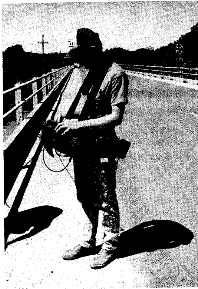
Figure 22. Chart-recording echo sounder being used with carrying case and battery belt.
