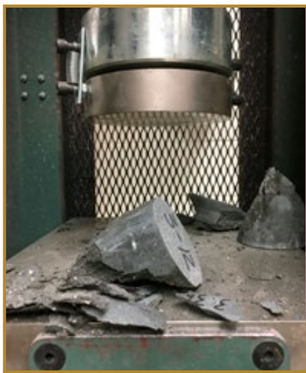
Figure 3: Brittle Failure of Cylinder after Compression Test
