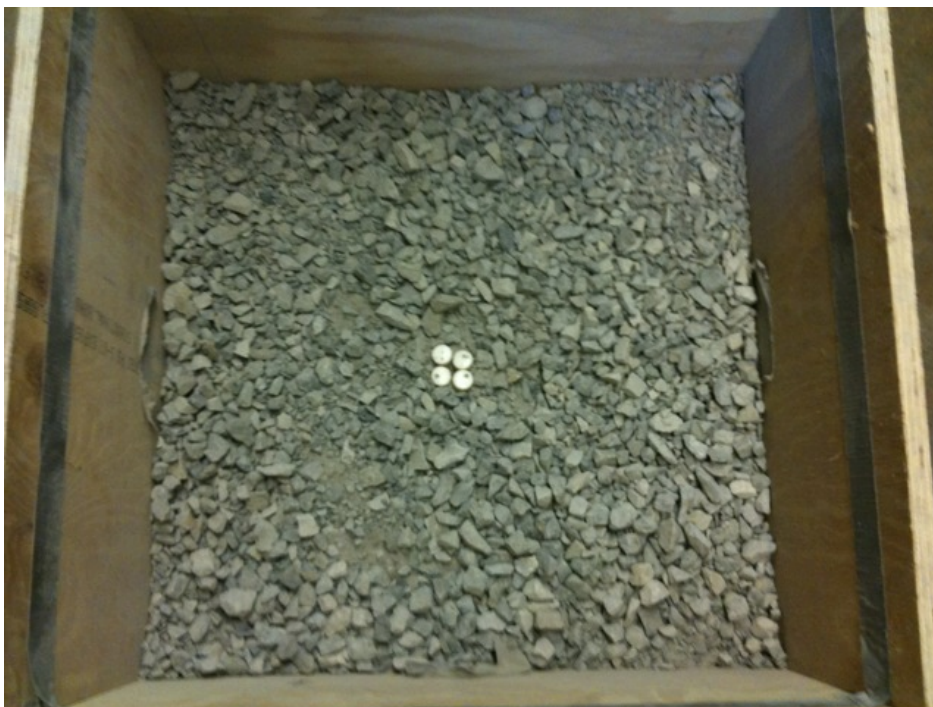
Figure 59. Photo. Tags located 12 inches (300 mm) from the bottom and 12 inches (300 mm) from the sides.
