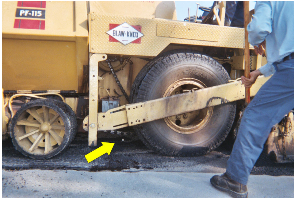
Figure 25. Photo. Encapsulated tag beneath paver.
