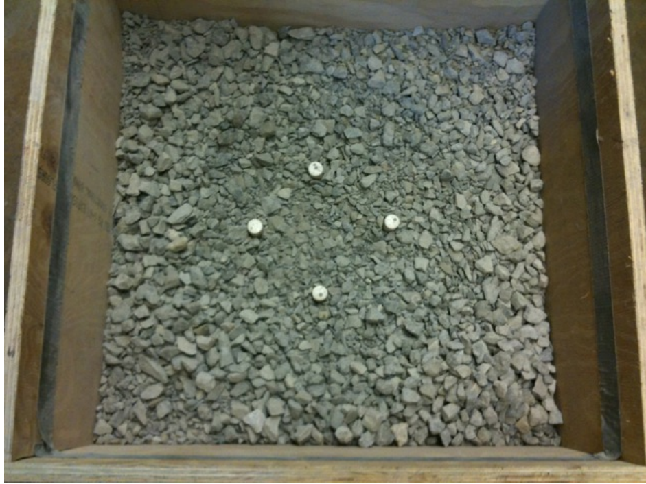
Figure 60. Photo. Tags located 8 inches (200 mm) from the top and 8 inches (200 mm) from the sides.
