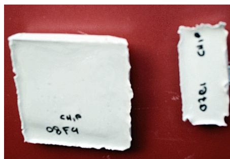
Figure 76. Photo. Encapsulated RFID tags before finish sanding (left: single patch, right: monopole).
