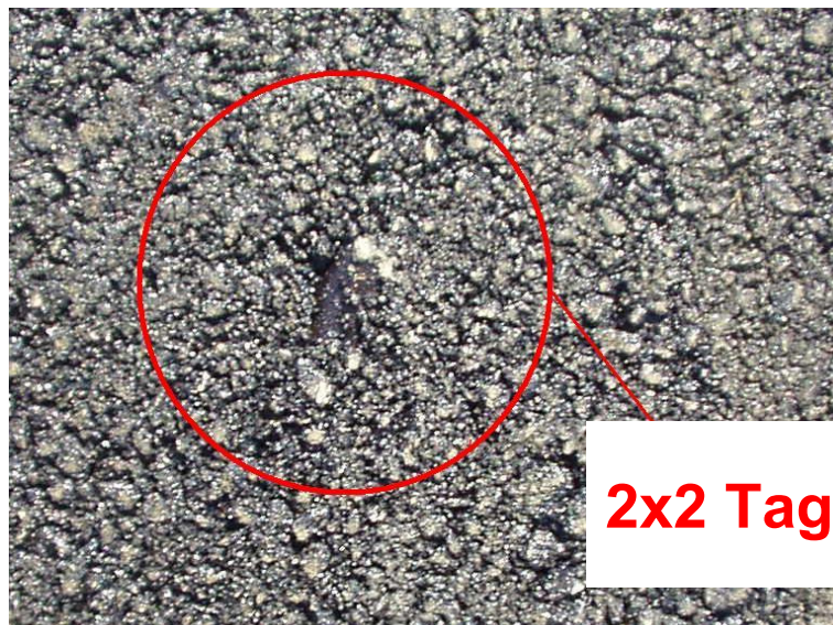
Figure 28. Photo. Examples of surfaced RFID tags in Lot EE.
