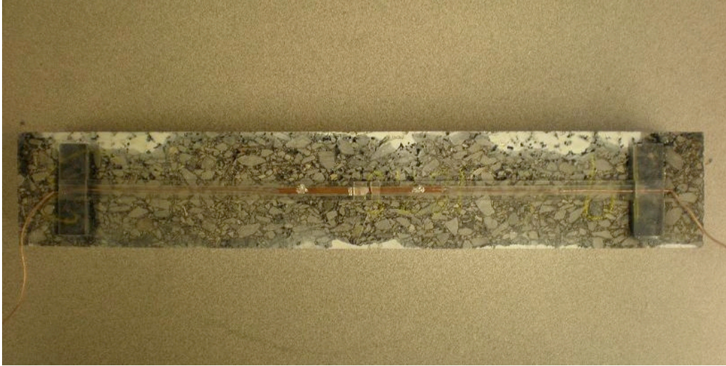
Figure 163. Photo. RFID tag glued to the asphalt beam.
