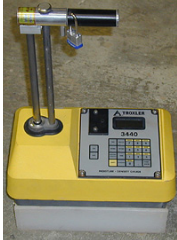
Figure 43. Photo. Troxler® Model 3440 nuclear density gauge.
