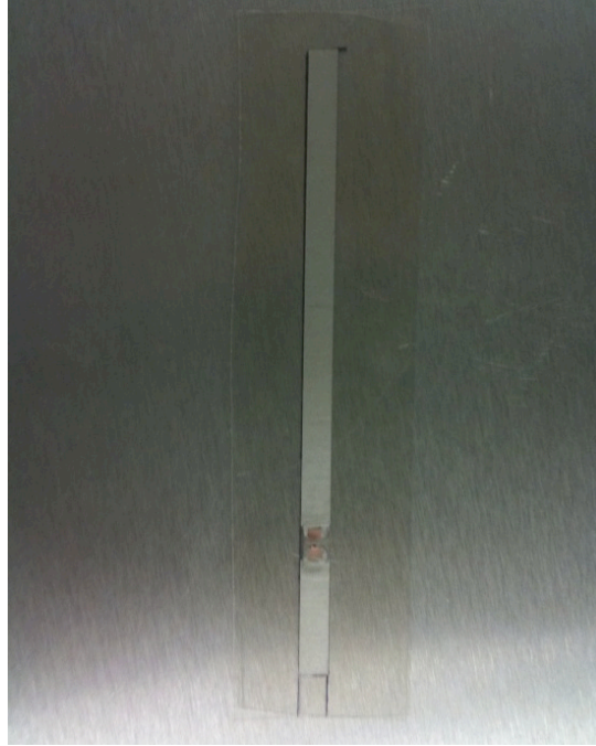
Figure 137. Photo. Silver dipole antenna with one side snipped at 0.8 inches (20 mm).
