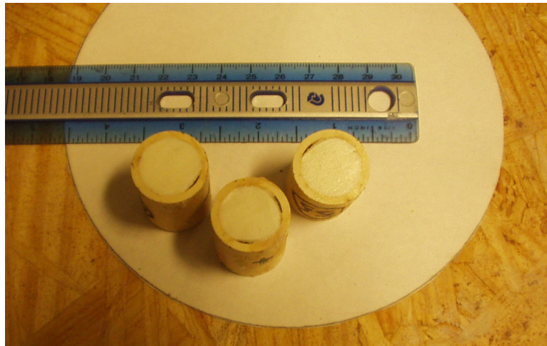
Figure 6. Photo. Voids between epoxy and CPVC pipe wall after filling at room temperature.
