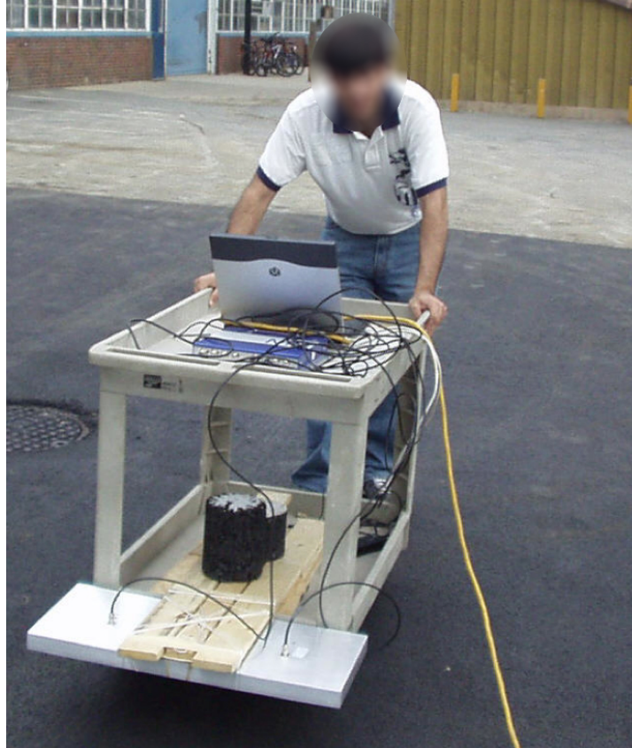
Figure 26. Photo. Hand cart for reading RFID tags in UMD parking lots with antenna in the lower position (10 inches above pavement surface).
