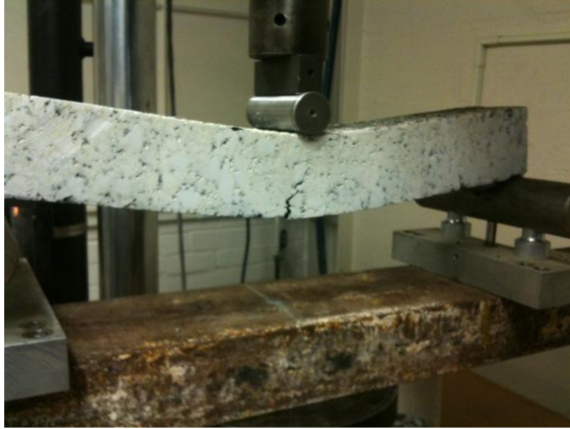
Figure 164. Photo. Crack propagation when the RFID tag stopped reading.
