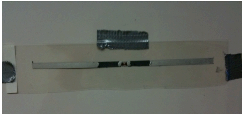
Figure 139. Photo. Silver and carbon dipole antenna.
