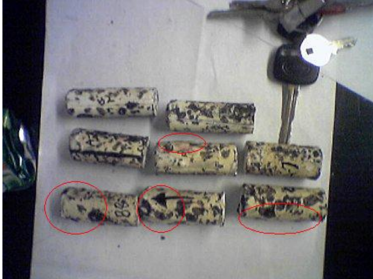
Figure 10. Photo. Post-mortem examination of tags retrieved from compacted HMA with bulges in encapsulated tags circled.
