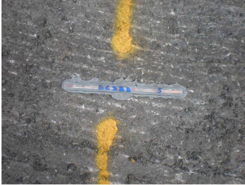
Figure 159. Photo. Close-up view of one of the encapsulated tags.
