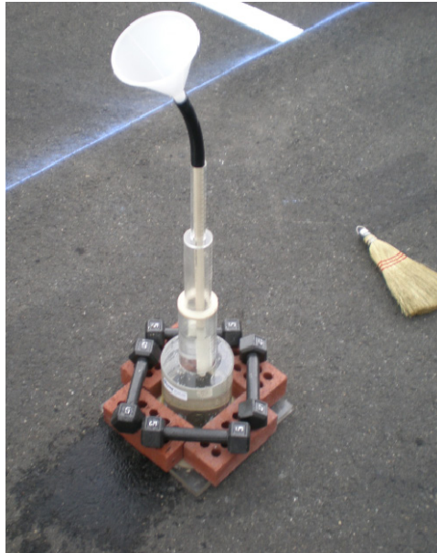
Figure 52. Photo. In-place permeability test setup.
