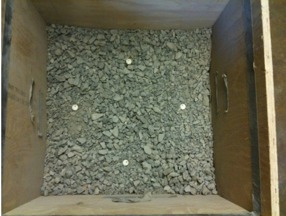
Figure 58. Photo. Tags located 8 inches (200 mm) from the bottom and 4 inches (100 mm) from the sides.
