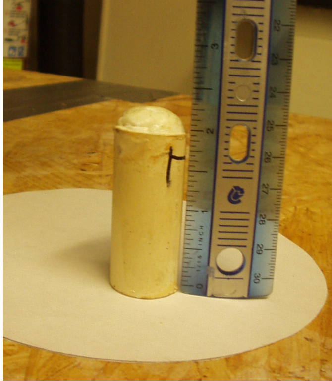
Figure 8. Photo. Extrusion of epoxy from end of pipe after oven curing.
