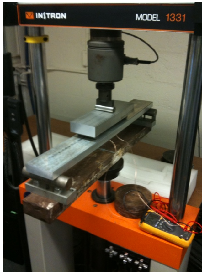
Figure 141. Photo. Thin film test setup.
