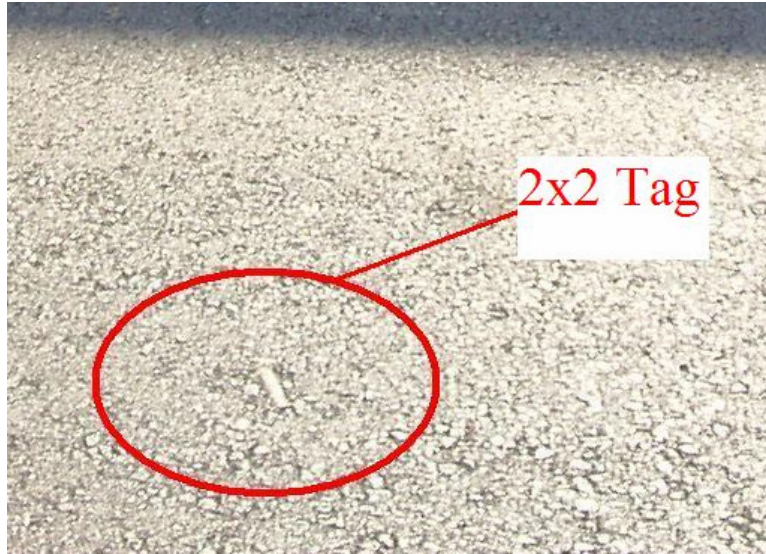
Figure 29. Photo. Worst-case example of surfaced RFID tag in Lot EE.
