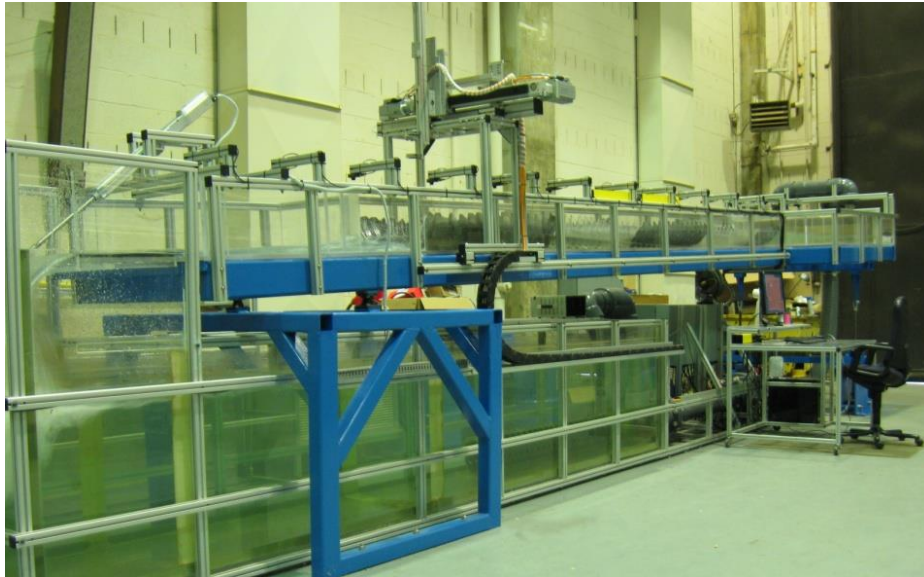
Figure 4. Photo. Fish passage culvert experimental flume.
