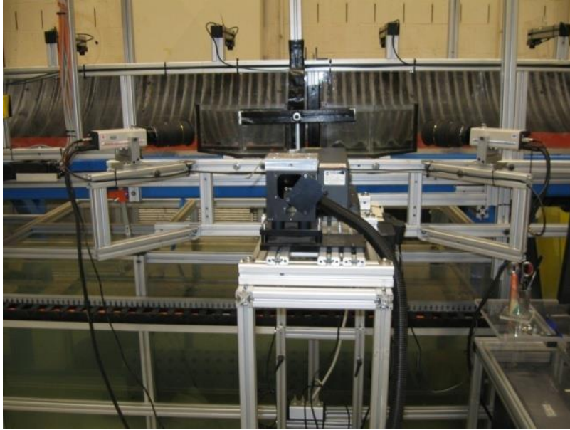
Figure 6. Photo. SPIV configuration.
