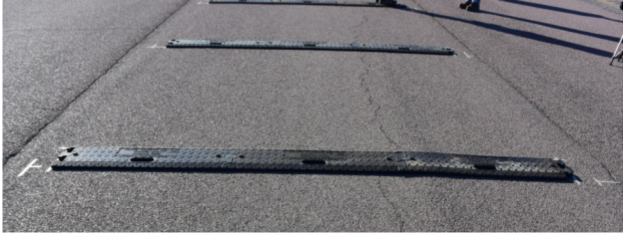
(a) Rumble Strips Layout – Viewed Longitudinally
