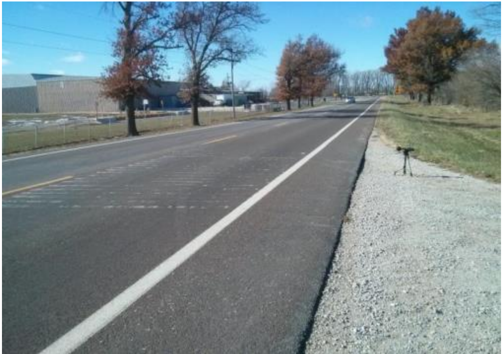
Figure C.4: Sound Meter Installation at 6 ft from Edge of Lane
