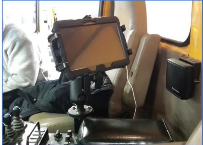
Tablet Computer in a WYDOT Plow Truck (Source: WYDOT)
