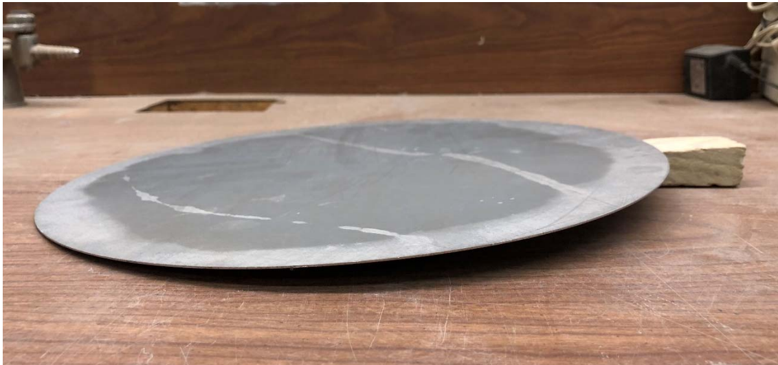
Figure 3 Example of a skewed reflector
