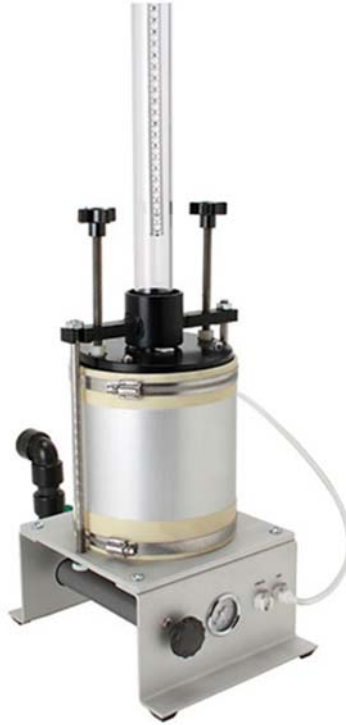
Figure 7 Falling head flexible wall permeameter
