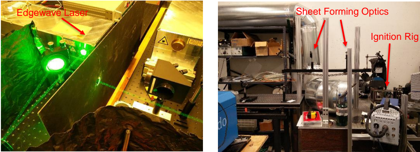
Figure 9 Edgewave pump laser (left) and dye laser with sheet forming optics, and the ignition rig
