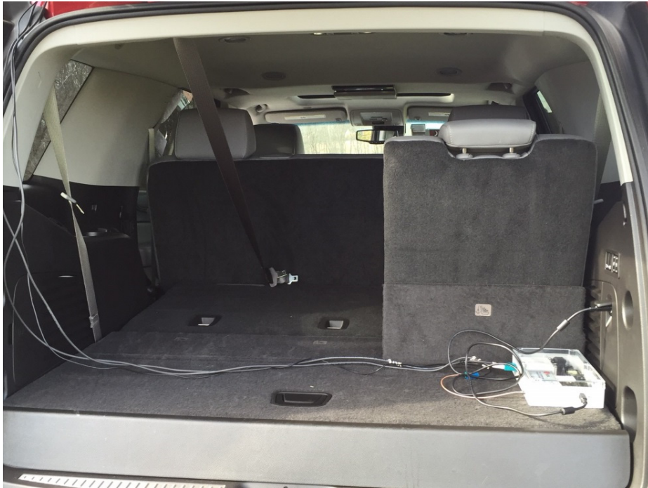
Figure 6-15. DSRC Radio Installed Temporarily in back of Oncoming Vehicles.
