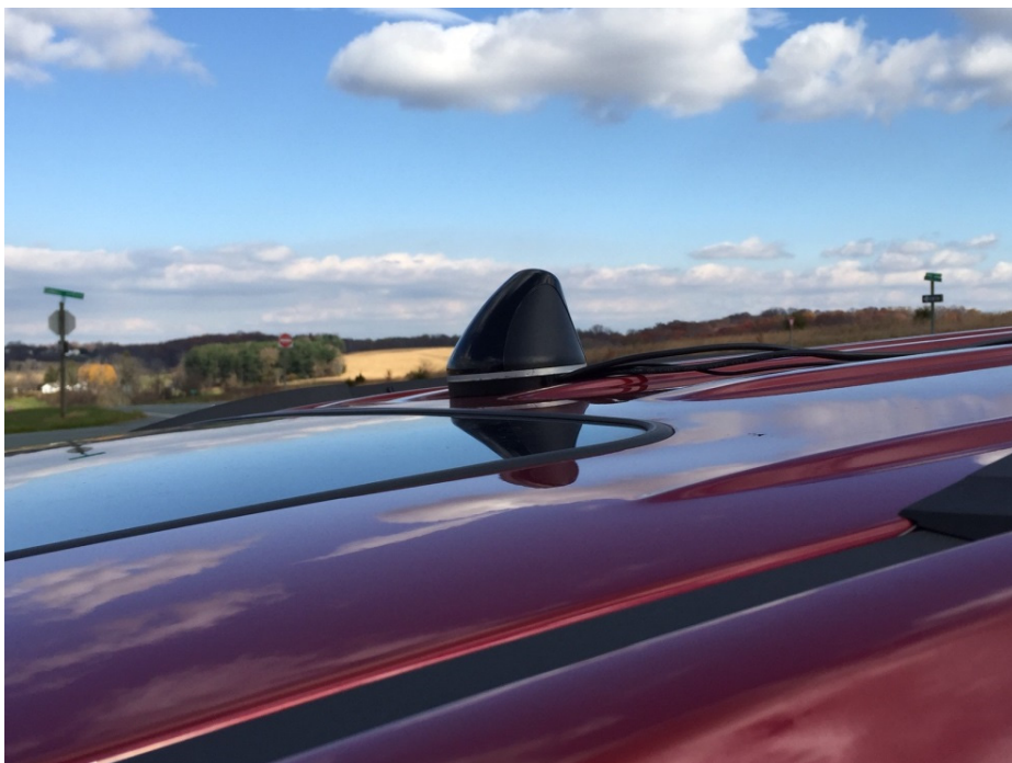
Figure 6-15. DSRC Radio Installed Temporarily in back of Oncoming Vehicles.
