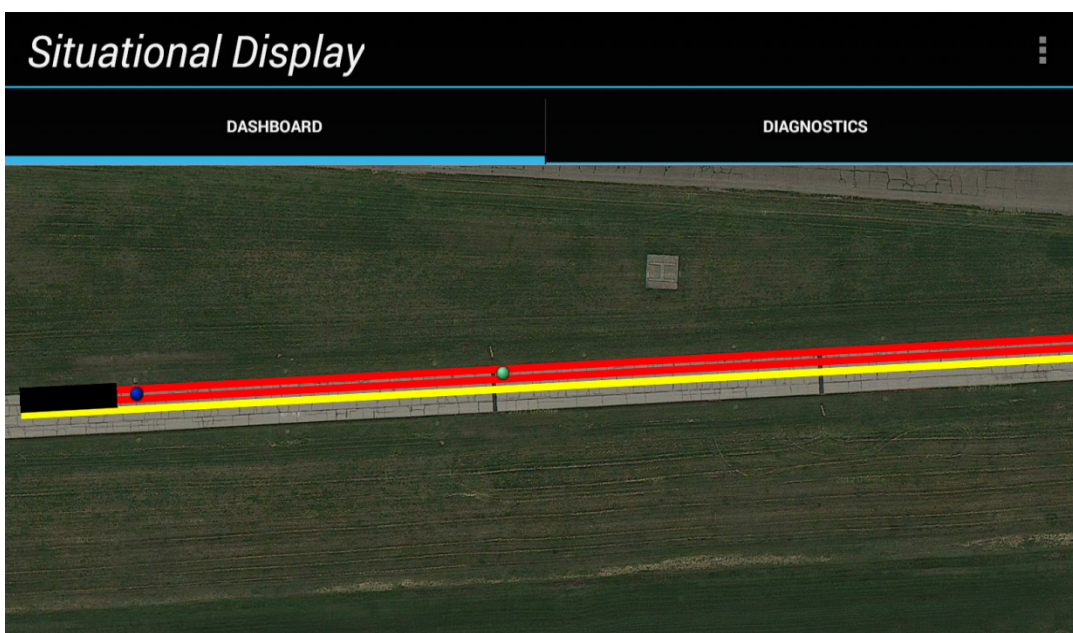
Figure 4-25. Display of Responder EVA Collision BSM and TIM Message Data showing the Closed Lanes as Red Lines, Reduced Speed Lane as Yellow Lines, the Responder Vehicle Blue Icon, Oncoming Vehicle Green Icon.
