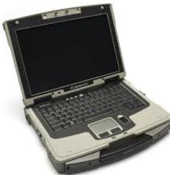
Figure 4-13. Panasonic Ruggedized Laptop used as the Responder Vehicle Computational Platform and User Interface.
