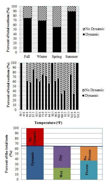
Figure 17. Graphs. Preliminary results—evidence of dynamic behavior by climatic information: classification by season (top), temperature (middle), and climate zone (bottom).
