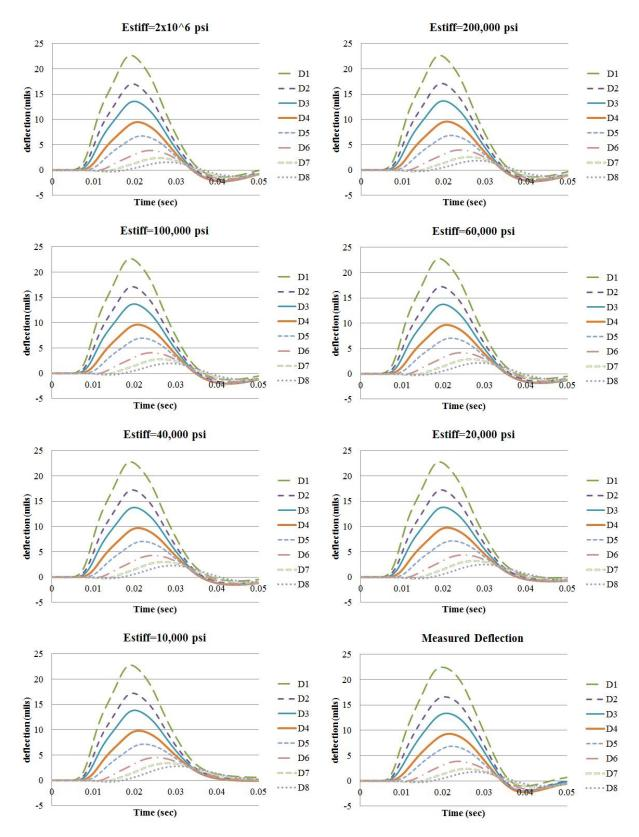
Figure 168. Graphs. Example time histories from ViscoWave-II with decreasing stiff layer modulus and measured sensor deflections for station 1.
