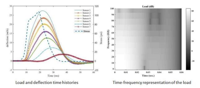
Figure 239. Graphs. Time-frequency content of the load for LTPP section 60565.
