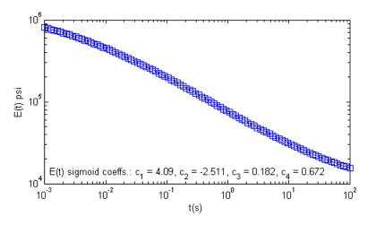
Figure 276. Graph. *E*(*t*) used to compute the deflection basin in examples 1 and 2.
