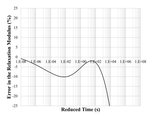
Figure 197. Graph. Error in the backcalculated master curve for LTPP section 350801.
