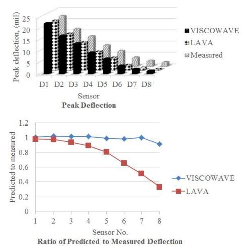
Figure 167. Graphs. Comparison of ViscoWave-II and LAVA solutions with measured deflections for station 1.
