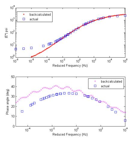
Figure 279. Graphs. Comparison of backcalculated and actual  $|E^*|$  and phase angle master curves for example 1.
