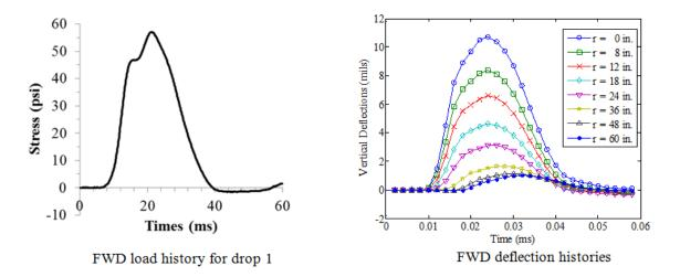
Figure 233. Graphs. Measured FWD load and time histories for LTPP section 300113.
