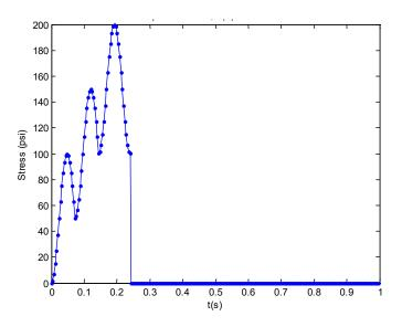
Figure 283. Graph. Stress history used in the constant frequency multiple pulse analysis.
