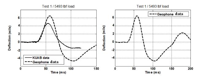
Figure 262. Graphs. Comparison between the filtered and treated seismometer data rendered by the device software and the integrated unfiltered geophone data (left); and integrated and filtered geophone data showing post-peak effects due to propagation of cumulative errors (right).
