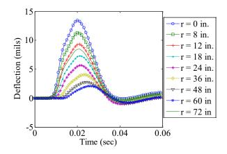
Figure 189. Graph. Measured FWD time histories for LTPP section 350801.
