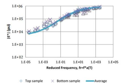
Figure 356. Graph. Laboratory-measured dynamic modulus at station 3 using 1.5- by 3.94-inch samples.
