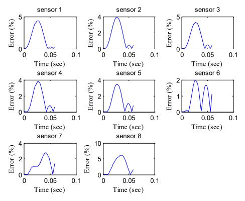
Figure 206. Graphs. Error in the backcalculated time histories by sensor for a pulse width of 50 ms.
