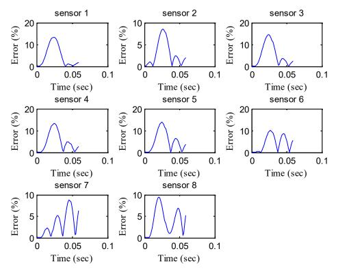
Figure 204. Graphs. Error in the backcalculated time histories by sensor for a pulse width of 40 ms.
