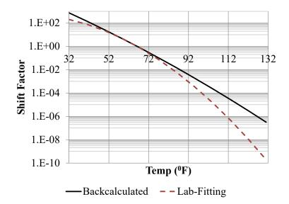
Figure 231. Graph. Backcalculated shift factors for LTPP section 6A806.
