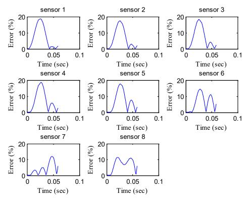
Figure 205. Graphs. Error in the backcalculated time histories by sensor for a pulse width of 45 ms.
