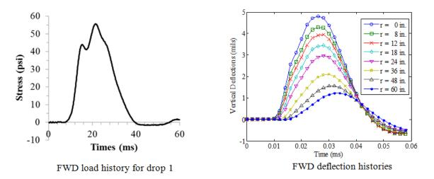
Figure 229. Graphs. Measured FWD load and time histories for LTPP section 6A806.
