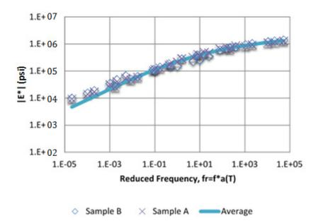
Figure 355. Graph. Laboratory-measured dynamic modulus at station 1 using 3.94- by 5.9-inch samples.
