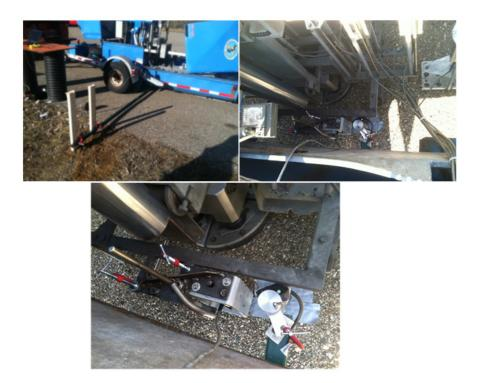
Figure 264. Photos. FWD test setup: view of the beam used for mounting the laser (top left), close-up view of mounted laser(top right), and view of laser sensor setup (bottom).
