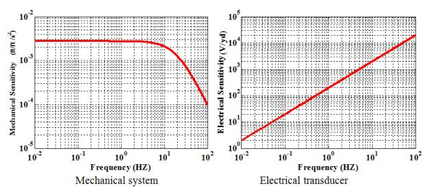
Figure 237. Graphs. Frequency response of geophone components.
