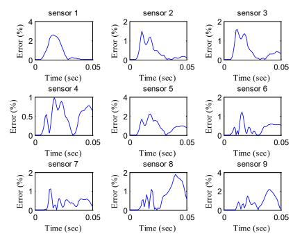
Figure 176. Graphs. Error in the backcalculated time histories by sensor—backcalculation of layer moduli only.
