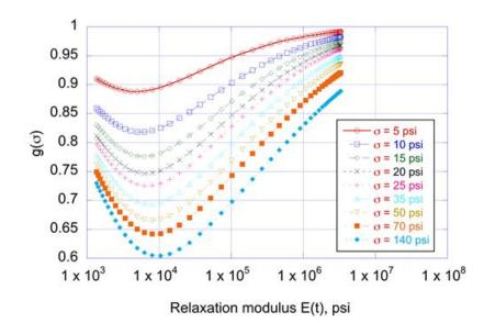
Figure 269. Graph. Variation of  $g(\sigma)$  with stress and E(t) of AC layer.
