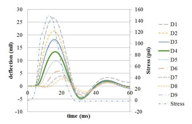
Figure 13. Graph. Example of time histories showing dynamic behavior for LTPP section 161020, station 1.
