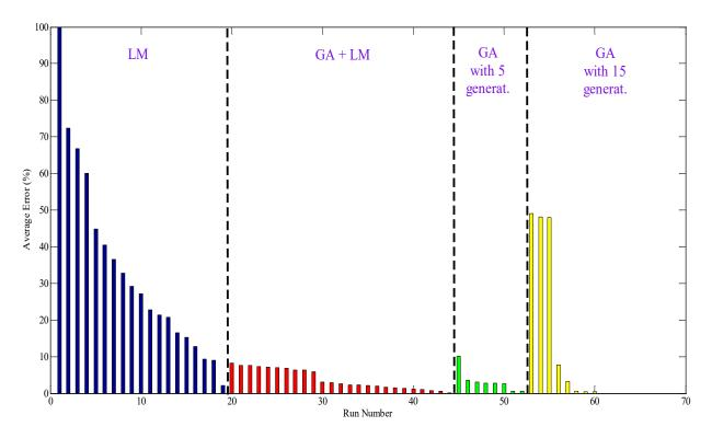
Figure 214. Graph. Average error in the backcalculated subgrade modulus for all runs.
