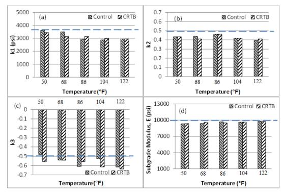
Figure 144. Graphs. Nonlinear elastic backcalculated unbound layer properties for control and CRTB mixes, using FWD data at different test temperatures.
