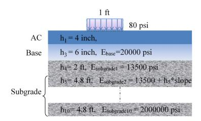
Figure 160. Diagram. Pavement structure with soils having *E*-values increasing with depth.
