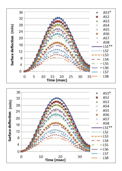
Figure 270. Graphs. Comparison of ABAQUS and LAVAN for nonlinear viscoelastic structure for the control mix where (top) LAVAN uses stress at r = 0, and (bottom) LAVAN uses stress at r = 3.5a.
