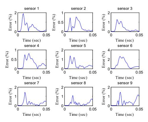
Figure 178. Graphs. Error in the backcalculated time histories by sensor—backcalculation of layer moduli and subgrade thickness.
