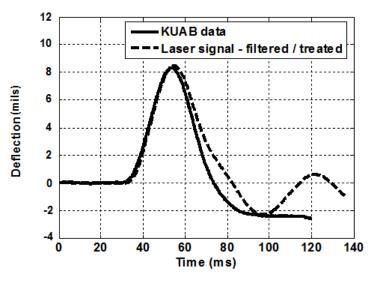
Figure 265. Graph. Comparison between the seismometer data rendered by the KUAB software and the filtered and treated laser data measured for a 9,500-lbf load.
