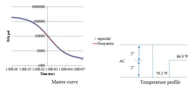
Figure 201. Graph and Diagram. AC layer parameters.
