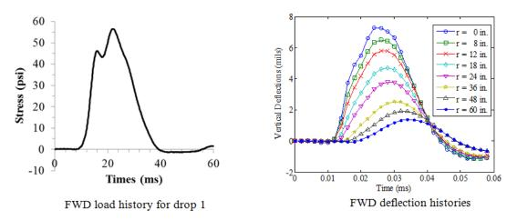
Figure 225. Graphs. Measured FWD load and time histories for LTPP section 6A805.
