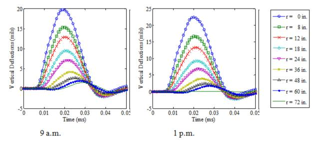
Figure 183. Graphs. Waverly Road FWD time histories for section1 collected at 9 a.m. and 1 p.m.
