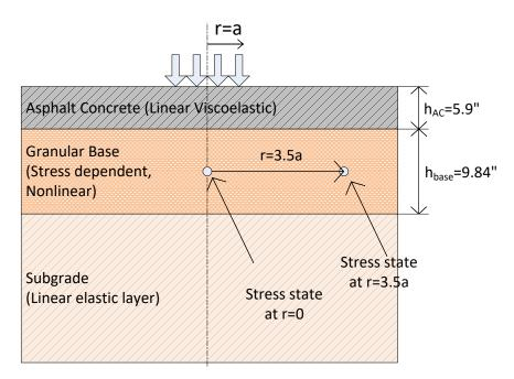
Figure 67. Diagram. Flexible pavement cross section for nonlinear viscoelastic pavement analysis.
