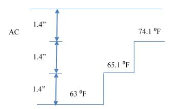
Figure 194. Diagram. Temperature profile for LTPP section 350801.
