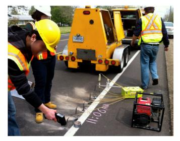
Figure 164. Photo. Illustration of temperature measurement at different depths of the pavement.
