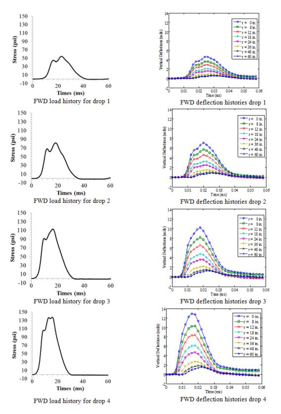
Figure 221. Graphs. Measured FWD load and time histories for LTPP section 10101.
