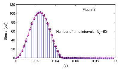
Figure 31. Graph. Discretization of stress history in forward analysis.
