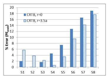
Figure 273. Graph. Percent error ( $PE_{peak}$ ) calculated using the peaks of the deflections for LAVAN-ABAQUS comparison (CRTB mix).
