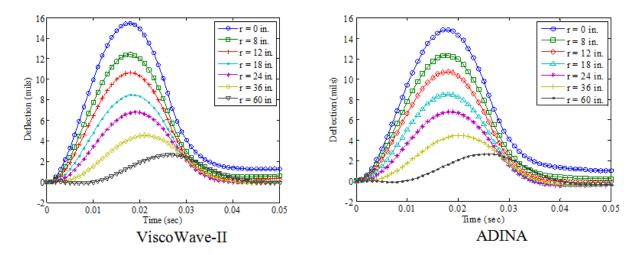
Figure 158. Graphs. Surface deflections of a layered viscoelastic structure with a half-space at high temperature simulated using ViscoWave-II and ADINA.
