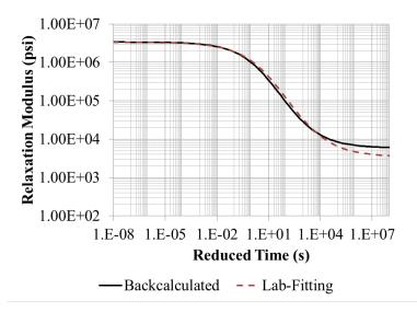
Figure 226. Graph. Backcalculated master curves for LTPP section 6A805.
