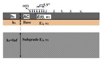
Figure 30. Diagram. Typical flexible pavement geometry for analysis.
