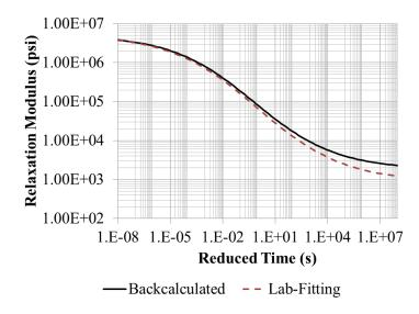
Figure 234. Graph. Backcalculated master curves for LTPP section 300113.
