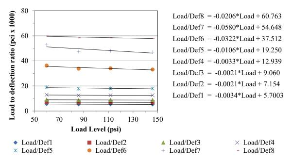
Figure 236. Graph. Load-to-deflection ratio for LTPP section 300113.
