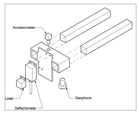
Figure 249. Diagram. Schematic of the designed fixture.
