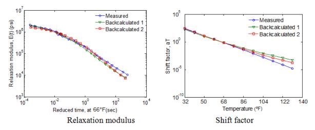
Figure 147. Graphs. Comparison of nonlinear viscoelastic backcalculated and measured E(t) and  $a_T(T)$  for LTPP section 10101.
