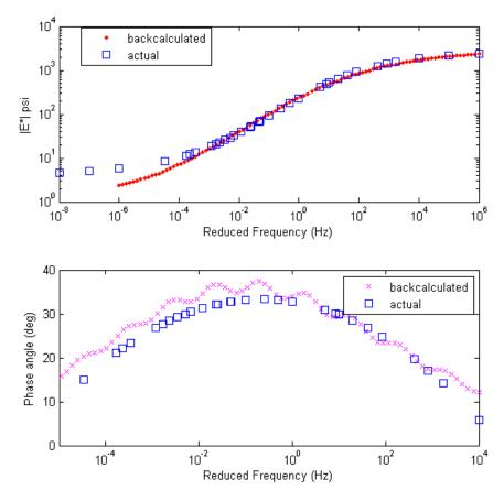
Figure 282. Graphs. Comparison of backcalculated and actual  $|E^*|$  and master curves for example 2.
