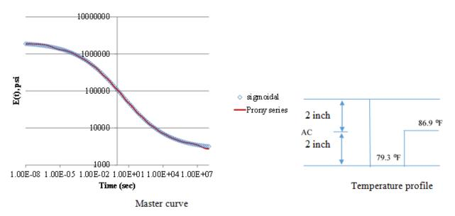
Figure 209. Graph and Diagram. AC layer master curve and temperature profile.
