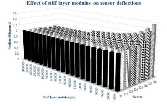
Figure 169. Graph. Effect of stiff layer modulus on ratio of predicted to measured sensor deflections for station 1.
