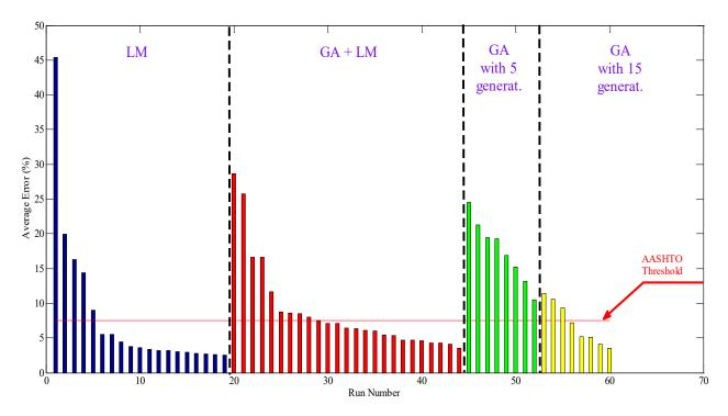
Figure 212. Graph. Average error in the backcalculated AC layer master curve for all runs.
