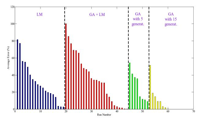
Figure 215. Graph. Average error in the backcalculated stiff layer modulus for all runs.
