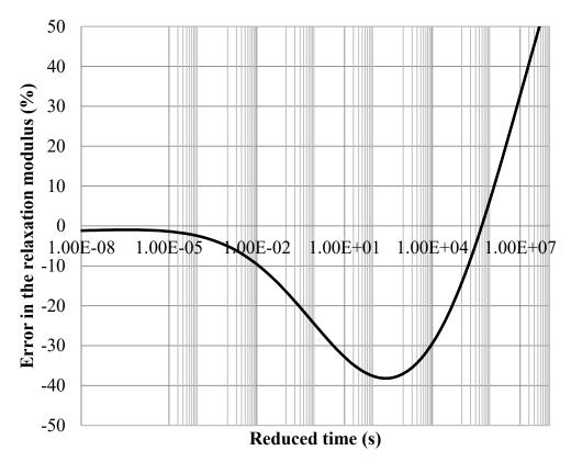
Figure 191. Graph. Error in the backcalculated master curve for LTPP section 350801.
