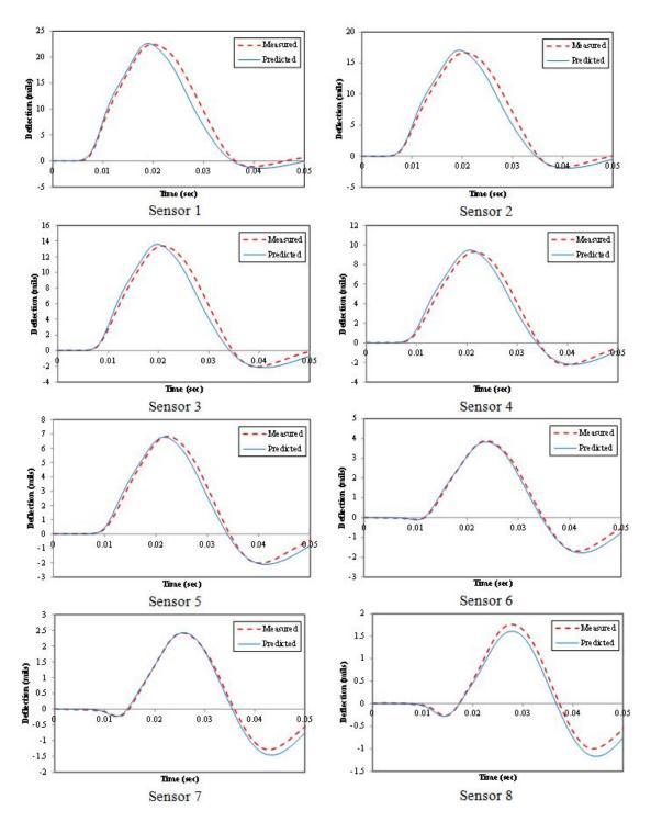
Figure 186. Graphs. Predicted versus measured deflection time histories by sensor for 1 p.m. test for Waverly Road.
