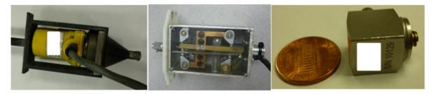
Figure 245. Photos. Geophone (left), seismometer (center), and high-accuracy piezoelectric accelerometer (right).
