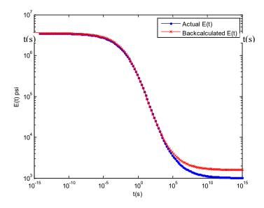
Figure 285. Graph. Result for backcalculated E(t) curve in example 1.
