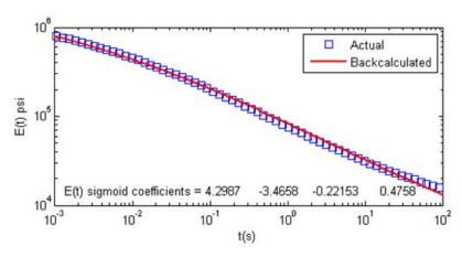
Figure 281. Graph. Backcalculated E(t) using multiple stress pulses.
