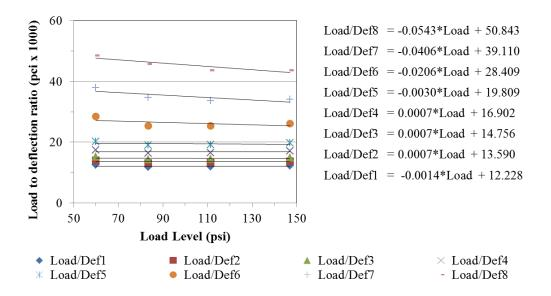
Figure 232. Graph. Load-to-deflection ratio for LTPP section 6A806.
