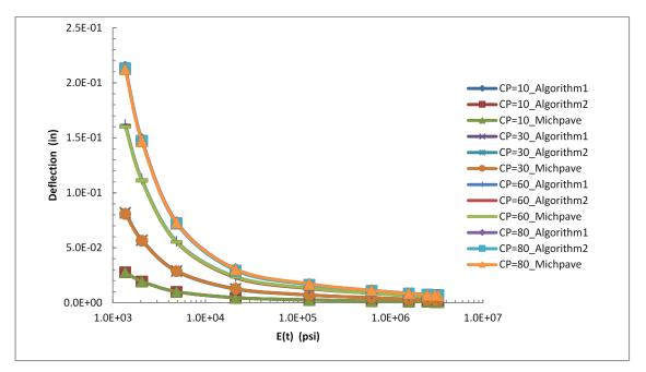
Figure 267. Graph. Results for multilayer nonlinear structure surface deflection at the center of the load (r = 0 inches).
