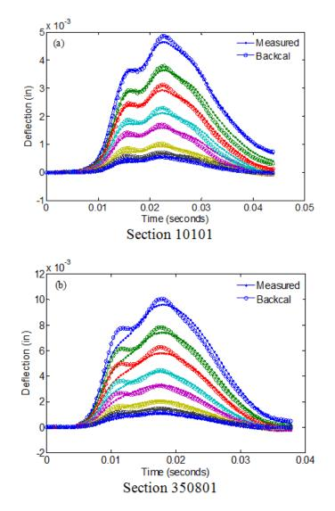
Figure 116. Graphs. Backcalculated and measured deflection time histories for LTPP sections 10101 and 350801.
