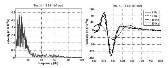
Figure 261. Graphs. Illustration of the windowing and filtering procedure and the observed effects on the raw velocity data: frequency content of the velocity signal (left) and effect of the selected cutoff frequency on the signal magnitude as a source of errors (right).
