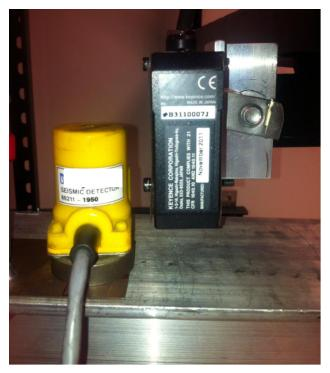
Figure 250. Photo. Geophone placed directly on beam next to laser sensor.
