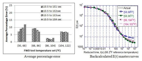
Figure 145. Graphs. Control mix backcalculation results from two-stage nonlinear viscoelastic backcalculation.
