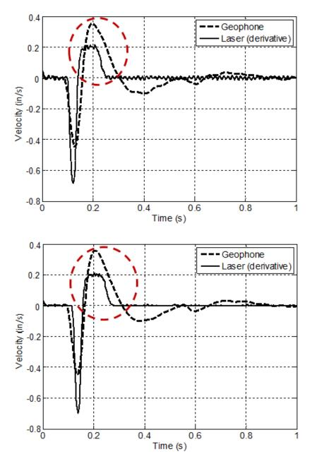
Figure 255. Graphs. Comparison of filtered geophone velocity data with the laser derivative output for test series 1.
