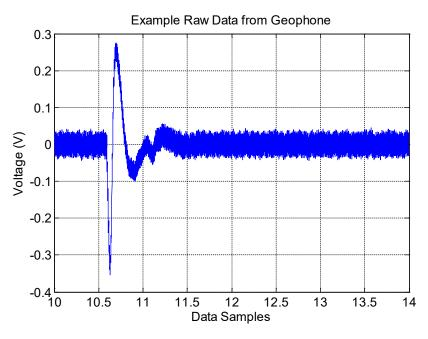
Figure 252. Graph. Example of raw data from geophone.
