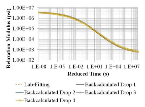
Figure 222. Graph. Backcalculated master curves for LTPP section 10101 from all the drops.
