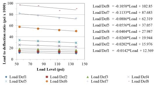
Figure 224. Graph. Softening behavior for LTPP section 10101.
