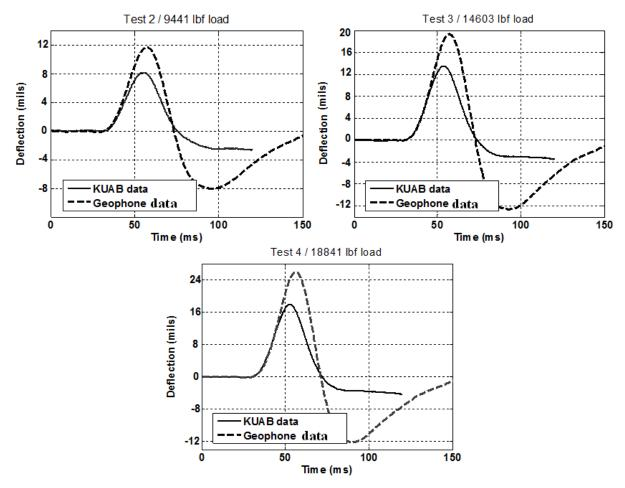
Figure 263. Graphs. Comparison between the filtered and treated seismometer data rendered by the device software and the integrated unfiltered geophone data at different load levels.
