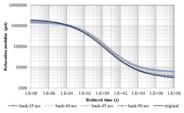
Figure 207. Graph. Backcalculation results of the AC master curve for different pulse widths.
