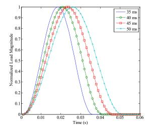
Figure 199. Graph. Simulated FWD load pulses with various durations.
