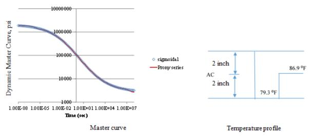
Figure 175. Graph and Diagram. AC layer master curve and temperature profile.
