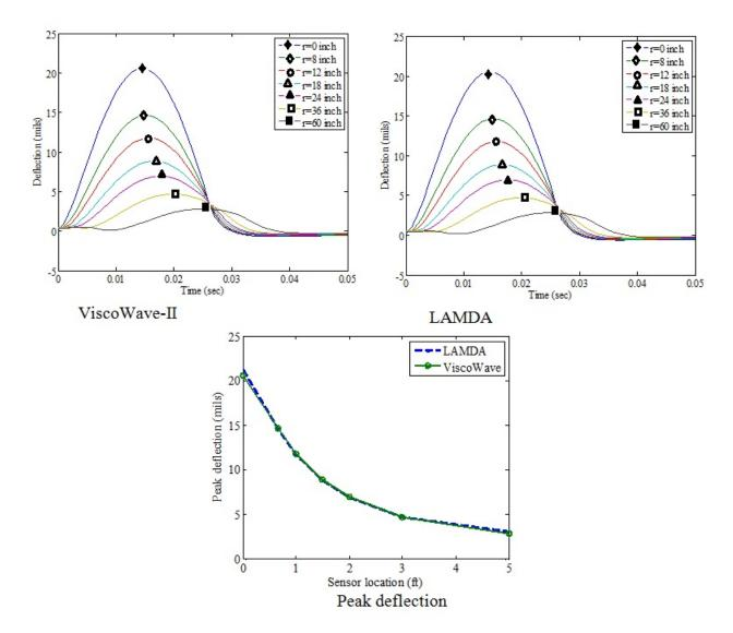
Figure 149. Graphs. Comparison of surface deflections of a layered elastic structure using ViscoWave-II and LAMDA.
