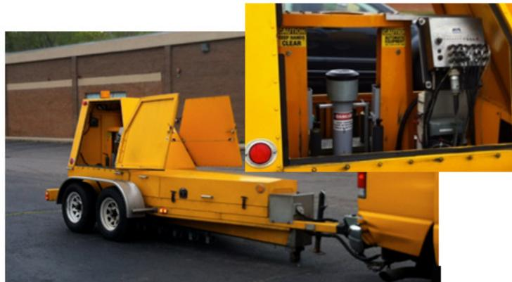
**Figure 163. Photos. FWD used during the field tests.**
