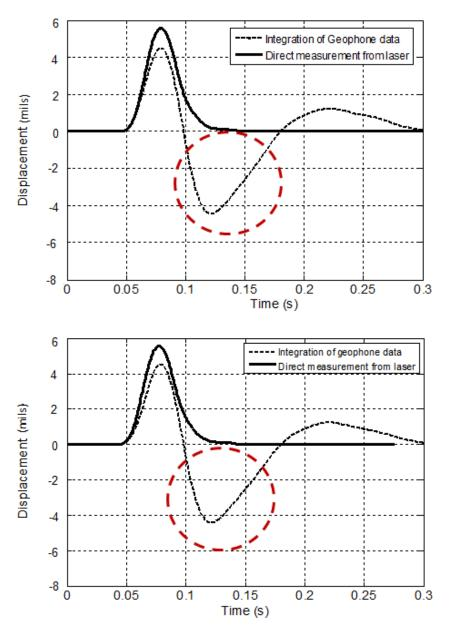
Figure 257. Graphs. Comparison of integrated geophone data with direct laser displacement output for test series 2.
