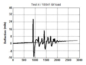
Figure 260. Graph. Example of numerical drift resulting from integration of raw geophone data.
