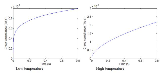
Figure 153. Graphs. Low- (left) and high- (right) temperature AC creep compliance curves used for ViscoWave-II simulation.
