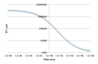
Figure 151. Graph. AC layer master curve for viscoelastic simulation.
