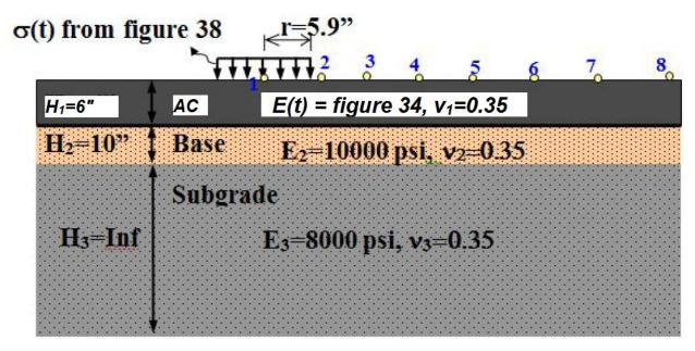
Figure 39. Diagram. Example problem geometry.
