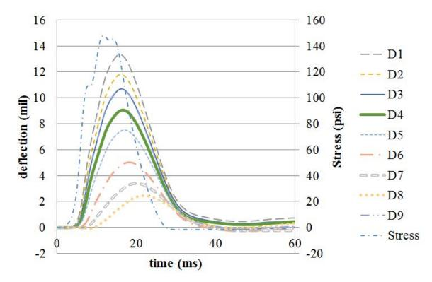
Figure 14. Graph. Example of time histories showing no dynamic behavior for LTPP section 169034, station 3.
