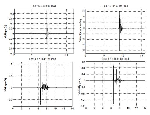
Figure 259. Graphs. Sample of recorded raw geophone data.
