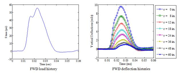
Figure 195. Graphs. Measured FWD load and deflection time histories for LTPP section 350801.
