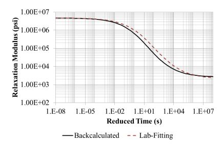
Figure 230. Graph. Backcalculated master curves for LTPP section 6A806.
