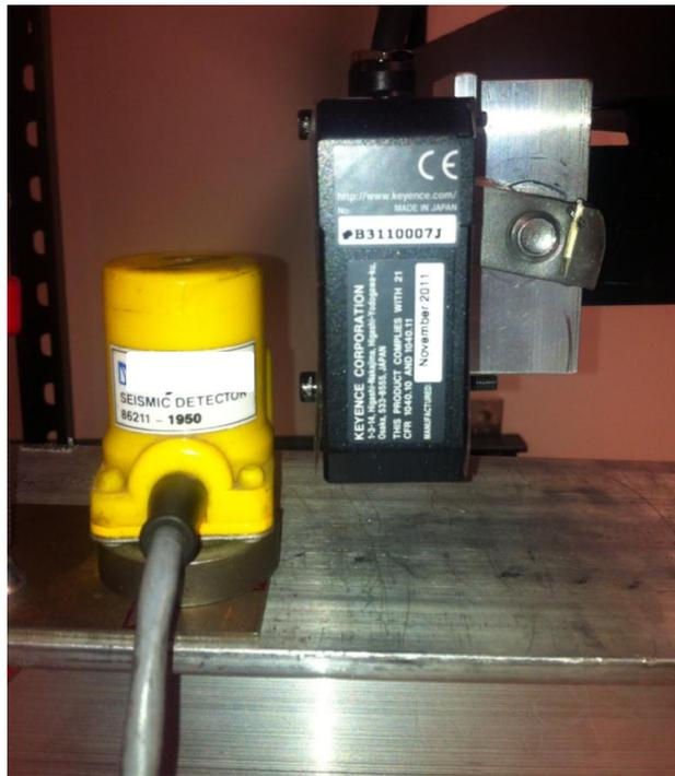
**Figure 250. Photo. Geophone placed directly on beam next to laser sensor.**
