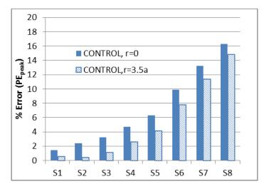
Figure 272. Graph. Percent error ( $PE_{peak}$ ) calculated using the peaks of the deflections for LAVAN-ABAQUS comparison (control mix).
