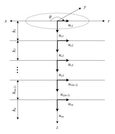
Figure 295. Diagram. Coordinate system for axisymmetric layers on a half-space.
