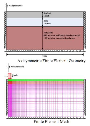
Figure 155. Diagrams. Axisymmetric FEM geometry (top) and FEM mesh (bottom) used for simulation of pavement response under FWD loading.
