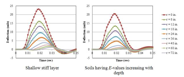
Figure 162. Graphs. Surface deflections of pavement structure with shallow stiff layer and soils having *E*-values increasing with depth.
