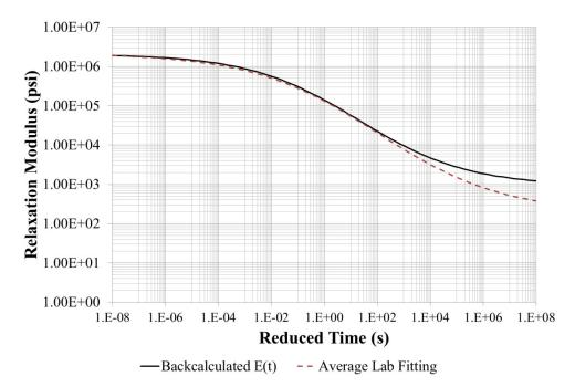
Figure 196. Graph. Backcalculation results of the AC master curve for LTPP section 350801.
