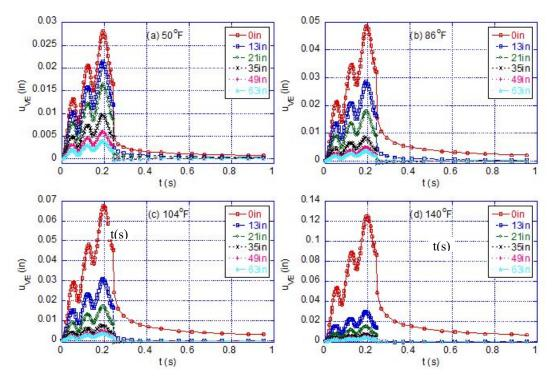
Figure 284. Graphs. Deflection at different sensors at different temperatures in example 1.
