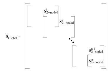
Figure 341. Equation. Construction of the global stiffness matrix for structures with a halfspace.
