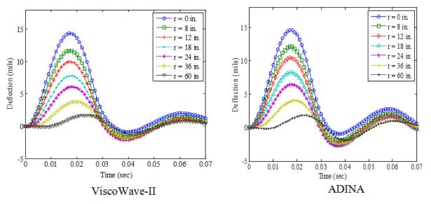
Figure 159. Graphs. Surface deflections of a layered viscoelastic structure with a bedrock at high temperature simulated using ViscoWave-II and ADINA.
