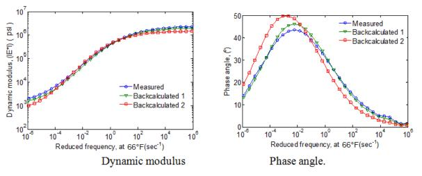
Figure 148. Graphs. Comparison of nonlinear viscoelastic backcalculated and measured  $|E^*|$  and phase angle for LTPP section 10101.
