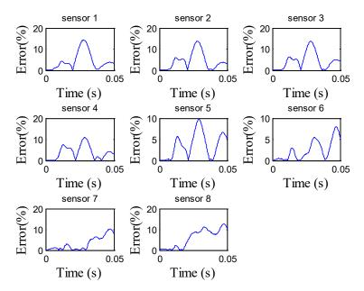
Figure 187. Graphs. Error in the backcalculated deflection time histories by sensor for 1 p.m. tests for Waverly Road.
