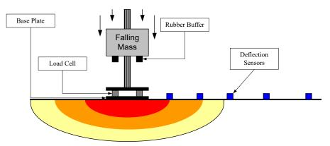
Figure 1. Diagram. FWD testing schematic.
