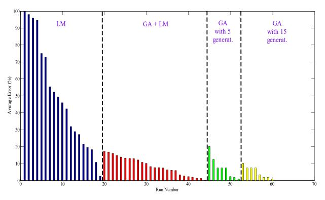
Figure 216. Graph. Average error in the backcalculated depth to the stiff layer for all runs.
