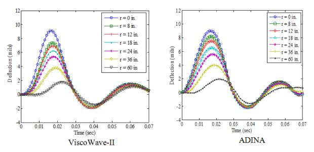
Figure 157. Graphs. Surface deflections of a layered viscoelastic structure with a bedrock at low temperature simulated using ViscoWave-II and ADINA.
