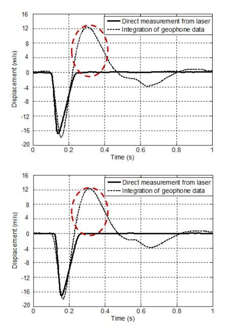
Figure 256. Graphs. Comparison of integrated geophone data with direct laser displacement output for test series 1.
