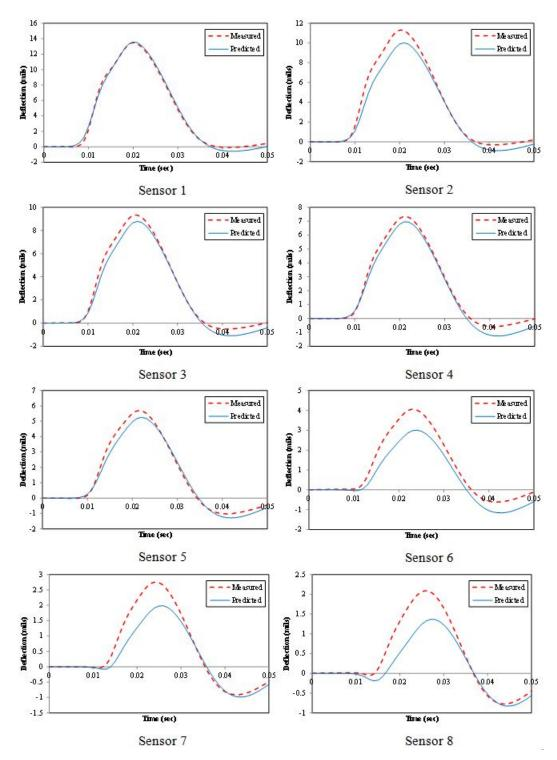
Figure 193. Graphs. Backcalculated versus measured deflection time histories by sensor for LTPP section 350801, station 1.
