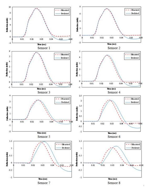
Figure 198. Graphs. Backcalculated versus measured deflection time histories by sensor for LTPP section 350801, station 8.
