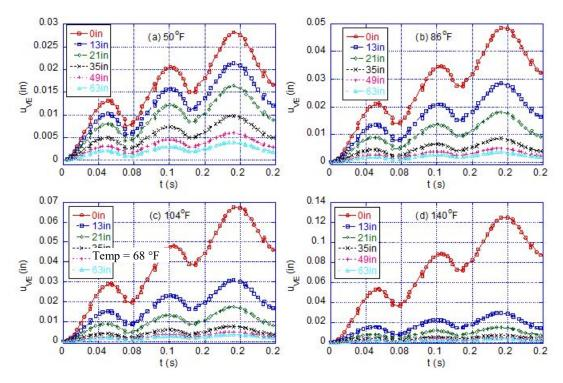
Figure 287. Graphs. Deflections at different sensors at different temperatures for example 2.
