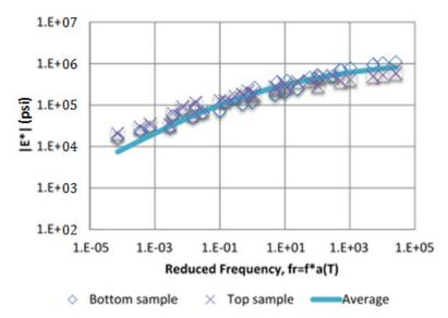
Figure 354. Graph. Laboratory-measured dynamic modulus at station 1 using 1.5- by 3.94-inch samples.
