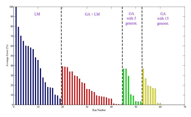
Figure 213. Graph. Average error in the backcalculated base layer modulus for all runs.
