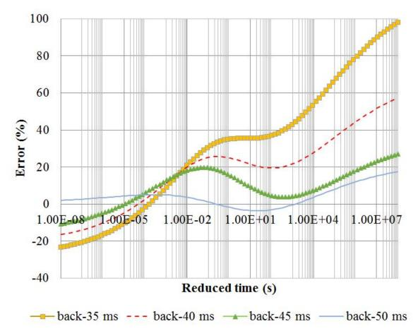
Figure 208. Graph. Error in the backcalculated master curve for different pulse widths.
