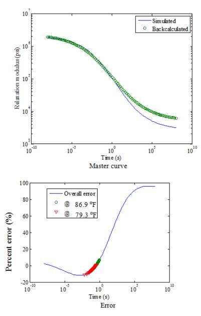
Figure 177. Graphs. Backcalculation results of the master curve—backcalculation of layer moduli only.
