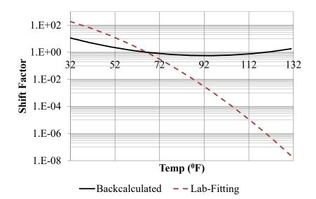
Figure 227. Graph. Backcalculated shift factors for LTPP section 6A805.
