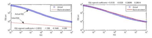
Figure 278. Graphs. *E(t)* and deflection history at the initial (left) and final (right) backcalculation stage in example 1.
