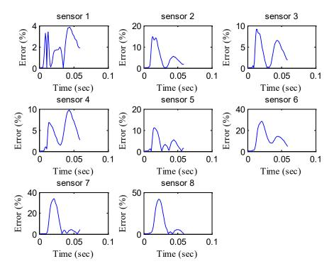
Figure 192. Graphs. Error in the backcalculated time histories by sensor for LTPP section 350801.
