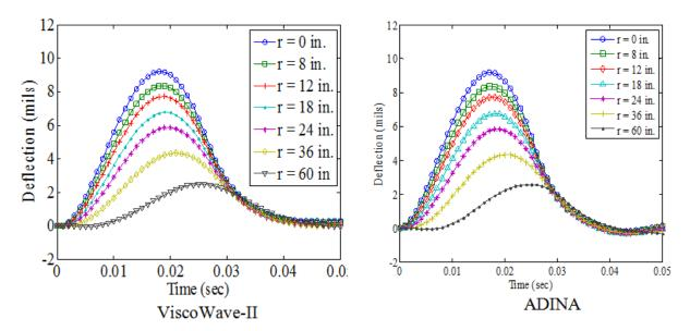
Figure 156. Graphs. Surface deflections of a layered viscoelastic structure with a half-space at low temperature simulated using ViscoWave-II and ADINA.
