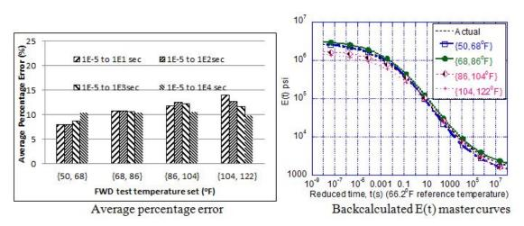
Figure 146. Graphs. CRTB mix backcalculation results from two-stage nonlinear viscoelastic backcalculation.
