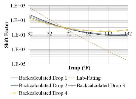
Figure 223. Graph. Backcalculated shift factors for LTPP section 10101 from all the drops.
