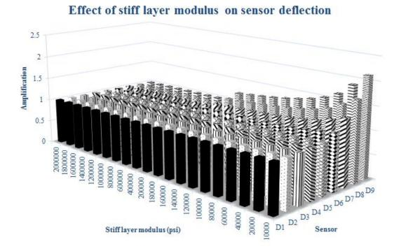
Figure 170. Graph. Effect of stiff layer modulus on predicted sensor deflection amplification for station 1.
