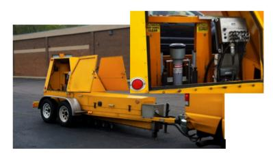
Figure 163. Photos. FWD used during the field tests.
