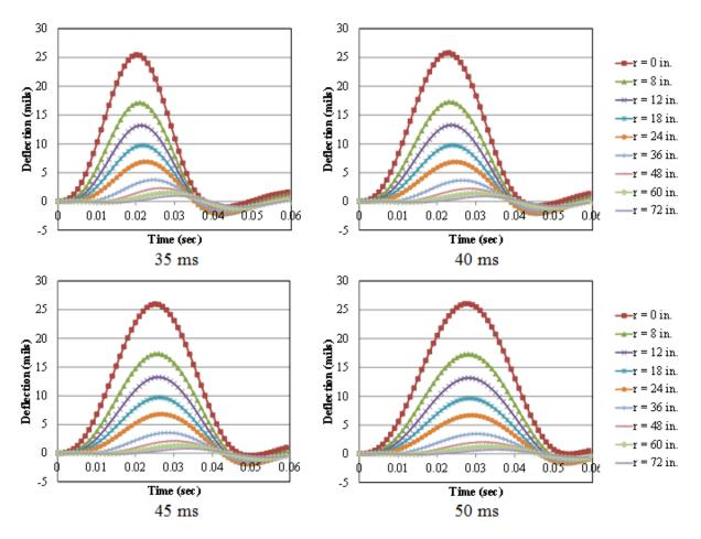
Figure 202. Graphs. Surface deflections of pavement structure for different widths of load pulses.
