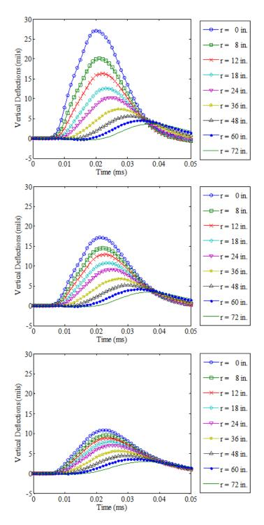
Figure 152. Graphs. Results from ViscoWave-II for viscoelastic simulations of thin (top), medium (middle), and thick (bottom)pavements.
