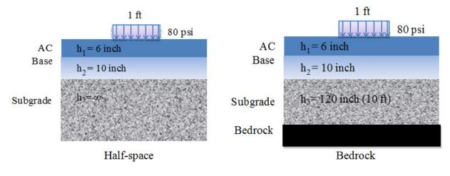
Figure 154. Diagrams. Schematic of the pavement structure with half-space (left) and bedrock (right).
