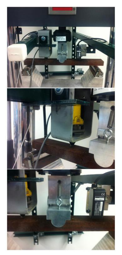
Figure 251. Photos. Test setup for mounted geophone and laser sensor.
