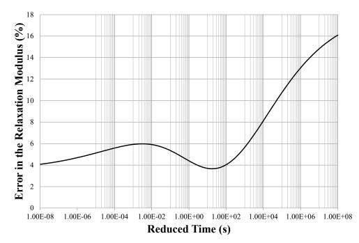
Figure 185. Graph. Error in the backcalculated master curve for Waverly Road.
