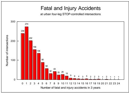
Figure 3. Accident Frequency Distributions at Urban, Four-Leg, STOP-Controlled Intersections
