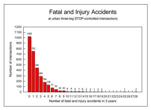
Figure 4. Accident Frequency Distributions at Urban, Three-Leg, STOP-Controlled Intersections
