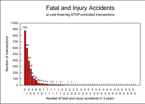
Figure 2. Accident Frequency Distributions at Rural, Three-Leg, STOP-Controlled Intersections
