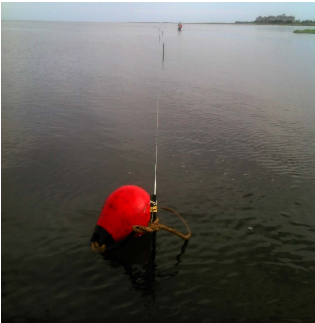
Figure 8. Image of baseline and datums for seabed inspection and close-plot metal detection survey (Nathan Richards/CSI).
