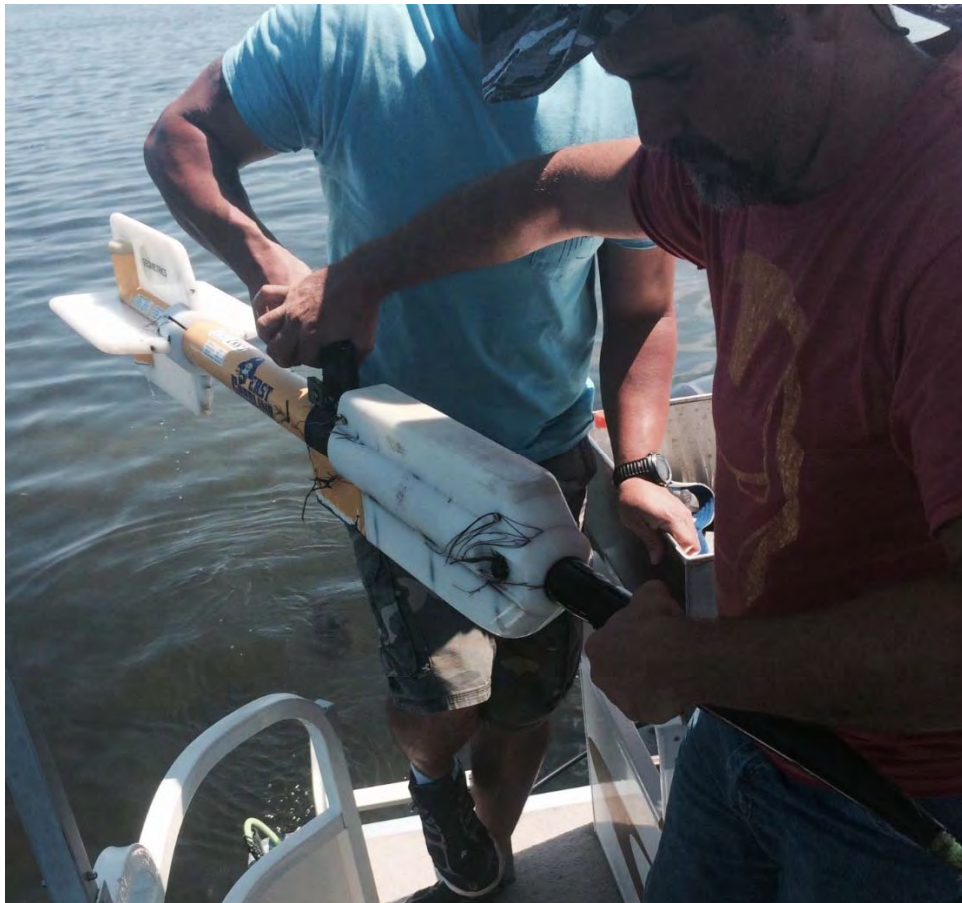
Figure 6. Jim Kinsella and Scott Rose retrieve Geometrics G882 magnetometer (Nathan Richards/CSI).
