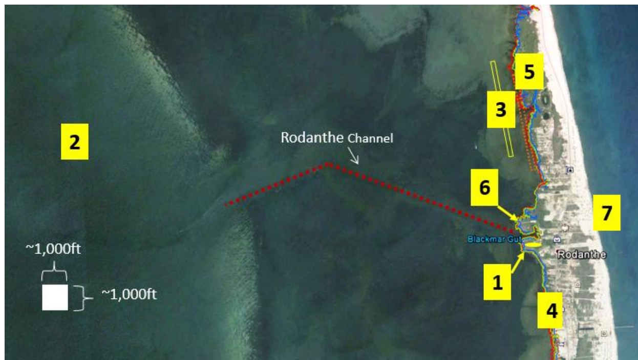
Figure 13. Disposal options considered in this study: 1) Existing Disposal Area, 2) Pamlico Sound Island, 3) Back-barrier Shoal, 4) Shoreline Nourishment and Reconstruction, 5) Marsh Accretion 6) New Local Area and 7) Distal Area.
