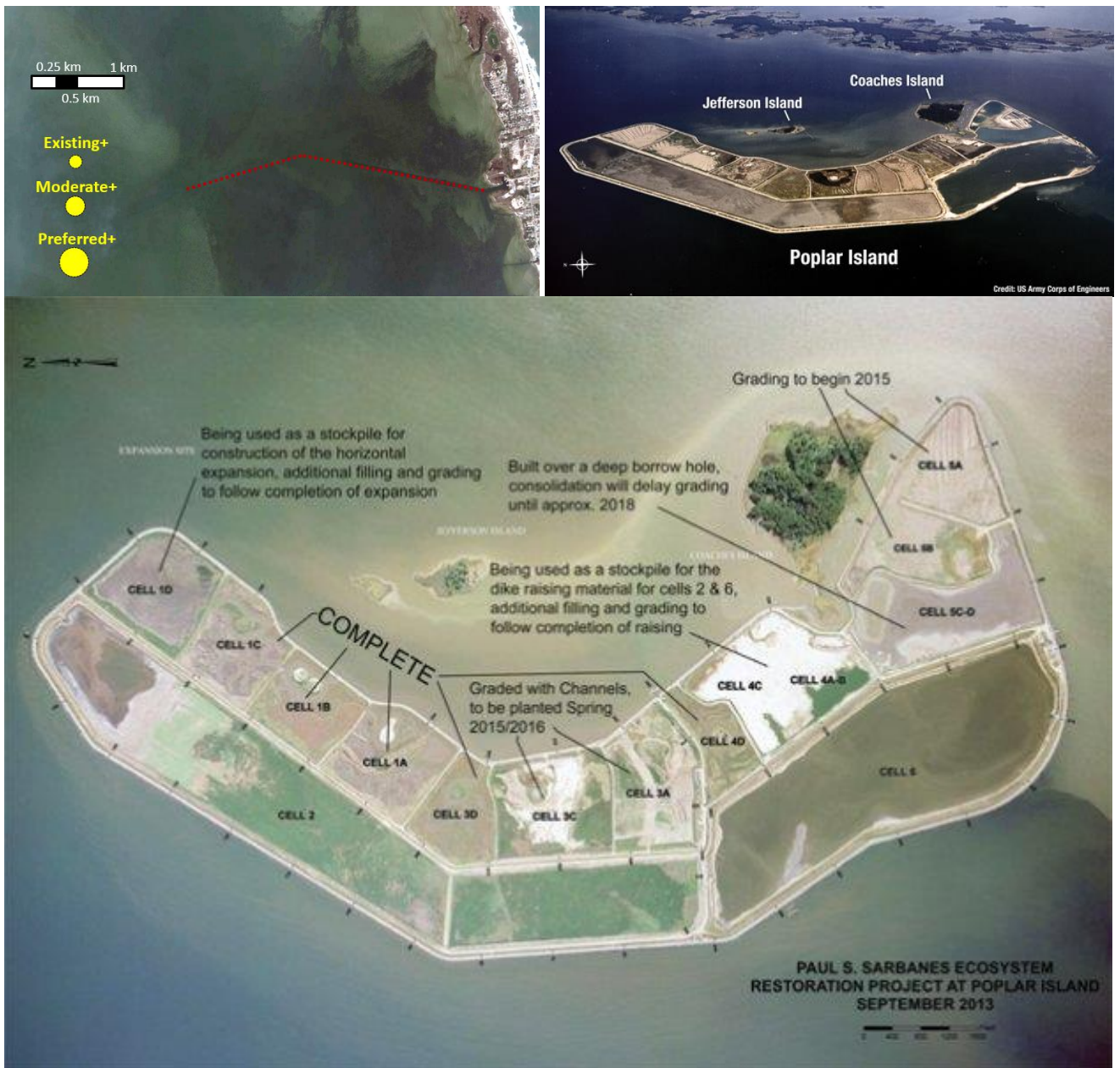
Figure 17. Potential size and approximate location of island (top left), oblique (top right) and annotated (lower) aerial example of a dredge spoil island (Poplar Island, MD). Image in top right from USEPA/USACE (2007b). Annotated image from Stinchcomb and Sharrett (2015). Of course, the location should not obstruct ferry traffic.
