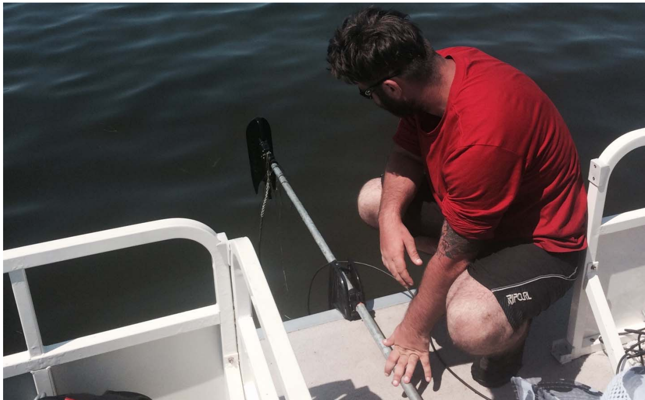
Figure 7. Adam Parker retrieves pole-mounted Tritech Starfish 650F sonar (Nathan Richards/CSI).
