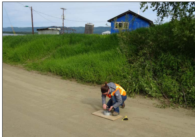
Figure 6. Abrasion of a sample to be tested using the Dustfall Column
