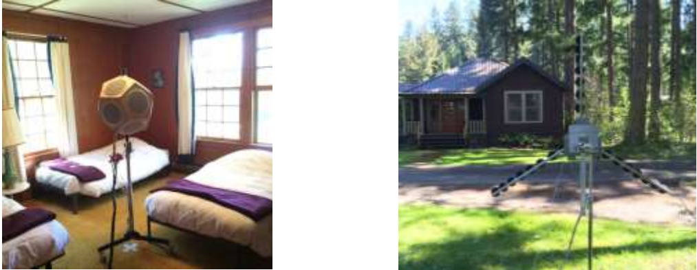
Fig. 1 (left) isotropic speaker inside the bedroom, (right) phased array of speakers outside.
