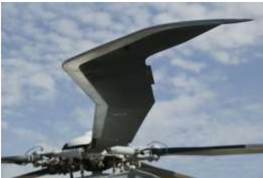
Figure 6.1. Blue Edge blade concept from Eurocopter (now Airbus Helicopters). [Ref. 6.1]
