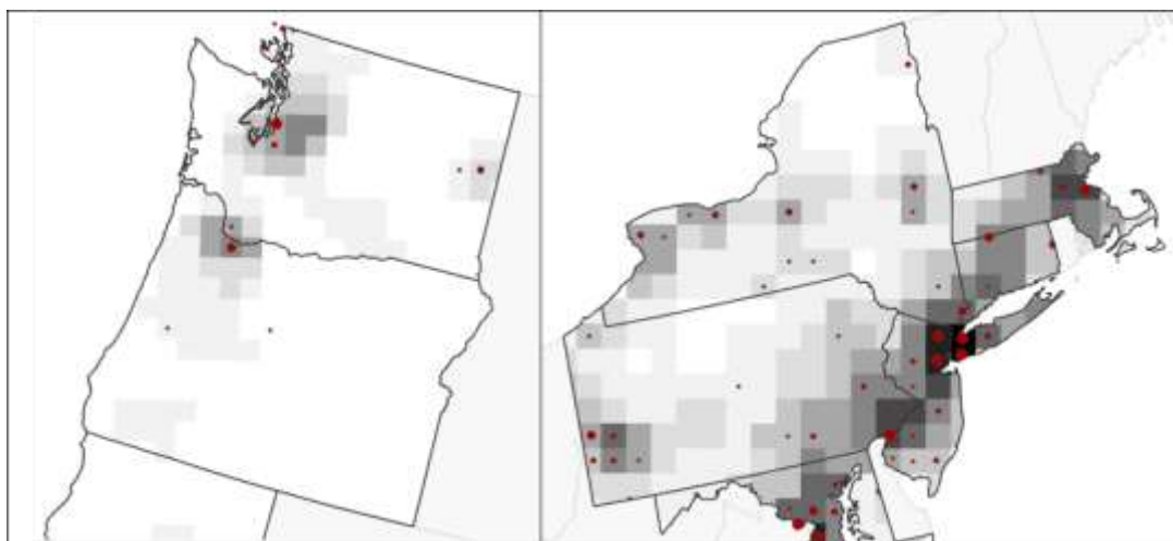
Figure 18.2. Relationship between population density and (2a) primary organic carbon (POC) emissions in January from aviation in the northwestern US and (2b) POC emissions in January from the aviation sector in the northeastern US. Total emissions per 36 x 36 km grid cell is represented by red graduated symbols, with larger symbols indicating higher emissions. Population density is represented by grayscale shading, with darker shading indicating higher population density.
