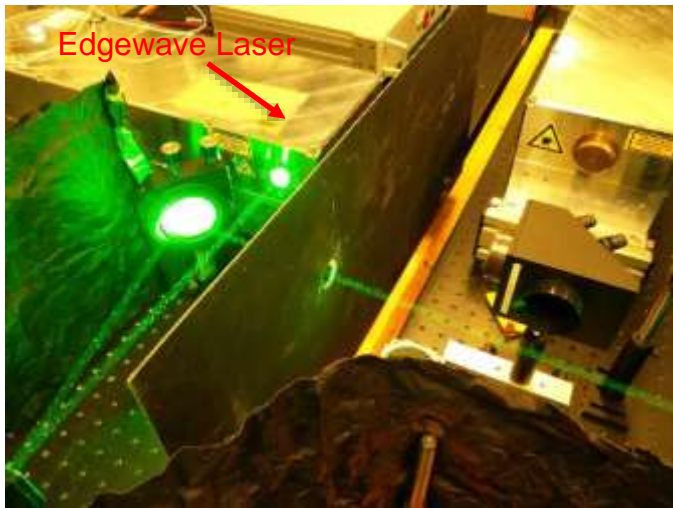
Figure 6. Edgewave pump laser (left) and dye laser with sheet forming optics, and the ignition rig
