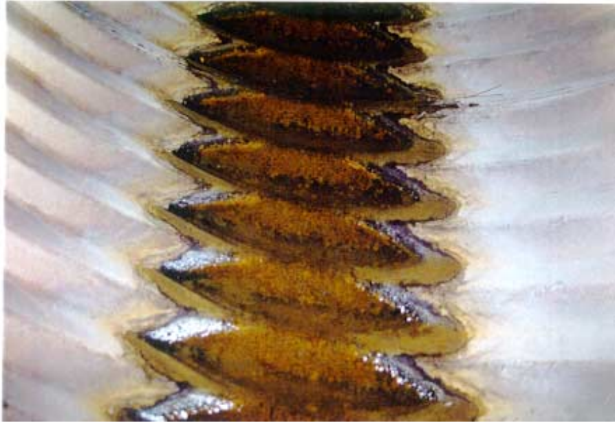
Figure 6. Aluminized Type 2 culvert after 5.5 years exposed to runoff with a pH of 2.5 to 3.5 (not from this study).
