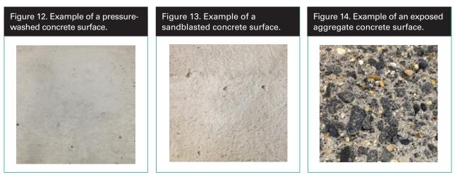
exposed aggregate surfaces leads to higher flexural bond strengths compared with other surface preparation methods applicable to precast concrete elements.
