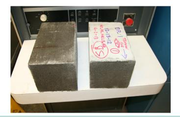
Figure 7. Typical failure modes exhibited in bond testing—failure location 2: partial substrate failure.
