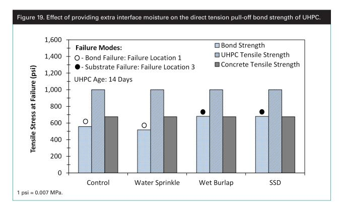
and SSD conditions enhance the tensile bond strength to the point that the failure occurred at the substrate rather than at the interface, as indicated by the concrete substrate tensile strength.
