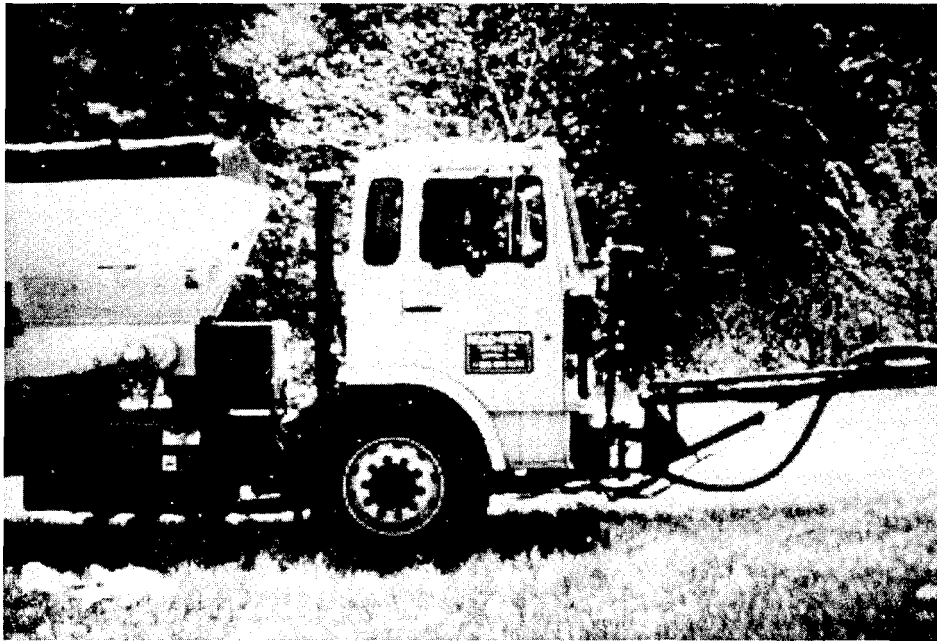
Figure 13. Wildcat Roadpatcher spray-injection device.
