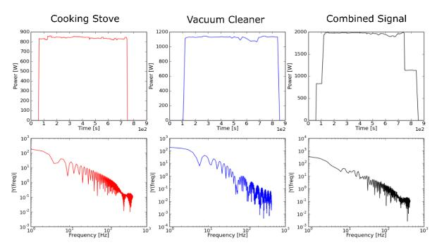
Figure 5.10: Once two device signals are combined they can then be analyzed in the frequency domain to better understand if the signals exhibit a specific characteristic pattern.
