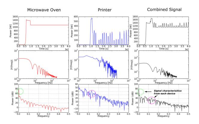
Figure 5.14: Column one displays the signal analysis for a microwave oven, column two for a printer, and column three for the sum of the two signals.
