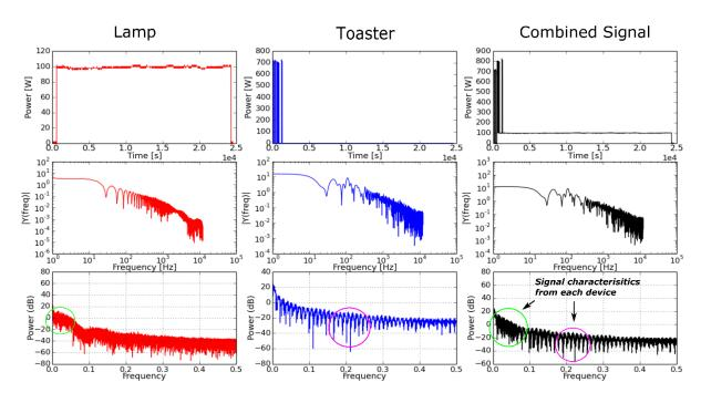
Figure 5.13: Column one displays the signal analysis for a lamp, column two for a toaster and column three for the sum of the two signals.
