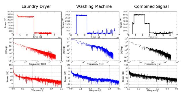
Figure 5.15: It can be seen in row three column three that it is not clear which devices make up the signal, so it is necessary to find an alternative method to identify device signatures.
