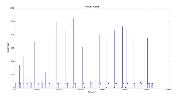
Figure 5.6: The power load data for a refrigerator is plotted to display differences between the power signatures of measured devices such as the water boiler in Fig. 5.3.
