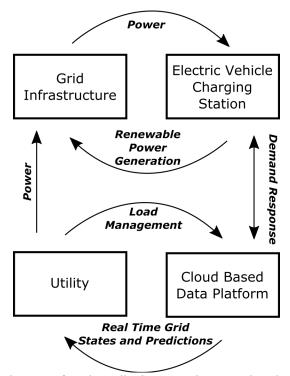
**Figure 3.1**: The system demand structure for a data collection system is presented. A cloud based platform will store and analyze data collected from a home, or business, in real-time, allowing for quick control decisions in demand response programs. One, or several EVCSs, can be analyzed within the urban environment by monitoring the amount of power consumed through the charging station using SPMs.
