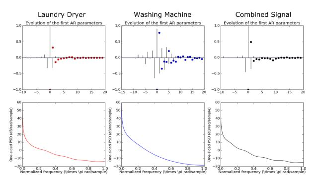
Figure 5.16: The AR parameters are plotted in the first row to show to what order they are significant for the respective devices. Defining the order of AR parameters is a necessary step in calculating the correlating PSD plot, which is shown in row two of the figure.
