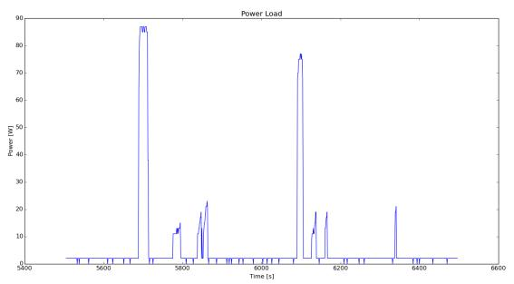
Figure 5.4: A closer look at the peaks within the plotted power data from a water boiler reveal unique transient changes, namely at the various power signal peaks.
