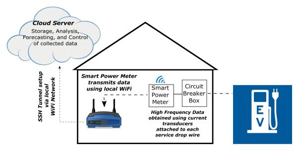
**Figure 3.4**: Utilizing preexisting WiFi connections within a home allow for a cost effective solution for data transmission. Circuit breaker boxes are usually located in a remote area of a building, so it is necessary to utilize a wireless connection to allow for a robust system to monitor and transmit data from a node. A secure SSH connection allows for safe and reliable transmission of data to a server in real-time. The pilot system structure was developed at the University of Hawaii.
