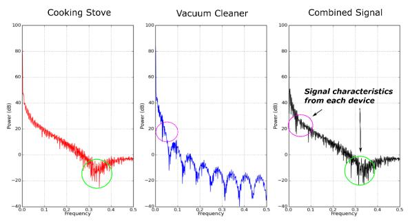
Figure 5.11: The implementation of PSD granted the capability to observe unique device signatures that are visible in an aggregated signal.
