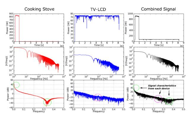
**Figure 5.12**: Column one displays the signal analysis for a cooking stove, column two for a LCD TV, and column three for the sum of the two signals. The green circle shows the location of a specific attribute of the cooking stove PSD signal in the aggregate, while the purple displays the attributes pertaining to the LCD TV.
