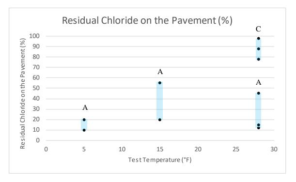
**Figure 2**. The range of residual chloride on the pavement surface (as %) after anti-icing, addition of snow and compaction, trafficking, and plowing, from this research effort (28°F on asphalt [A] and concrete [C] pavements) and from research by Muthumani et al. (2015) (5°F and 15°F) on asphalt (A) pavement.
