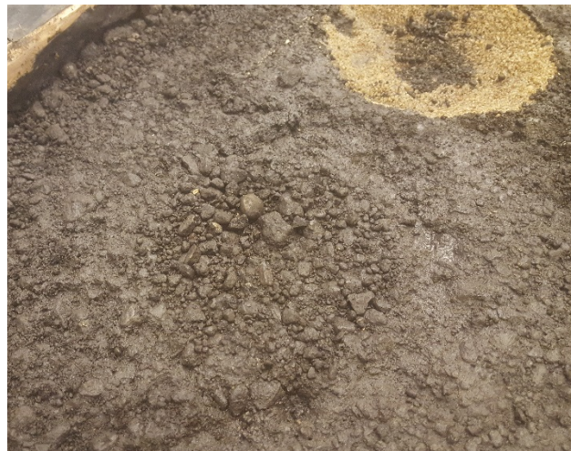
Figure 11. Washed fines after performing the permeability test.
