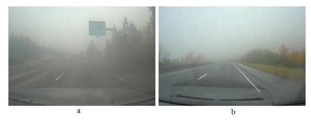
Figure 13 Near Fog: a) Only one road marking is visible, the sign is unreadable, surroundings and the horizon cannot be seen properly. b) Few road markings are visible, surroundings, traffic, and the horizon cannot be seen clearly.
