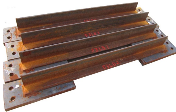
Figure 21: Angle-Plate Cross-Frame Specimens (McDonald and Frank 2009)
