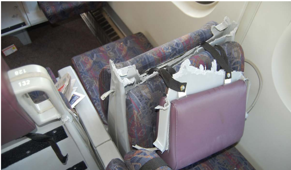
Figure 23. Broken Head Rests in Lower Level, Car #617
