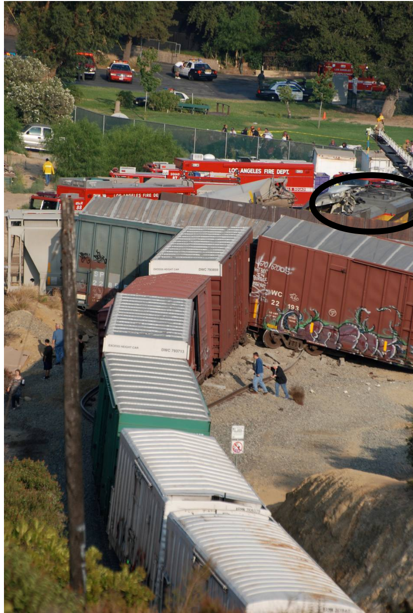
Figure 20. Freight Equipment Structural Damage
