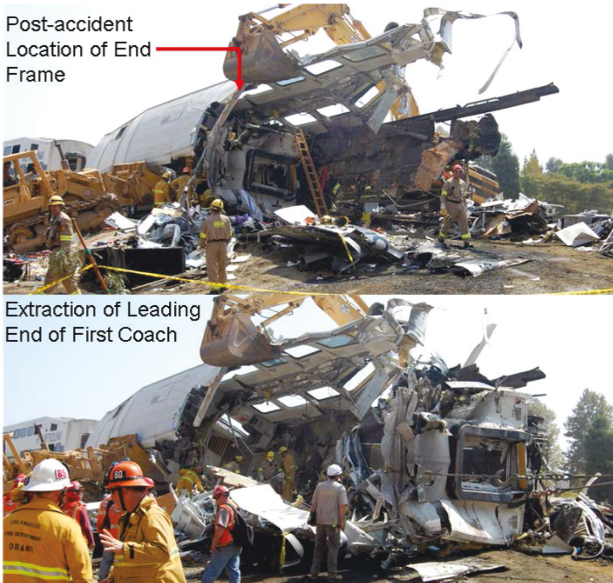
Figure 14. First Passenger Car Structural Damage
