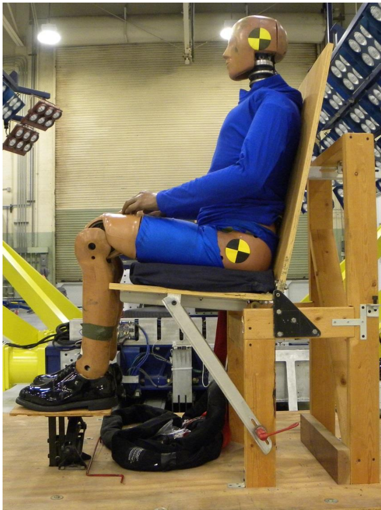
Figure 2. FAA Hybrid III on Wooden 1 G Seating Fixture
