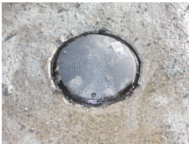
Figure 19. In-ground Parking Sensor in San Francisco
