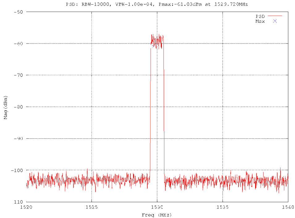
Figure 3-9: Type 1 Signal Captured during WSMR Testing @ 1530 MHz
