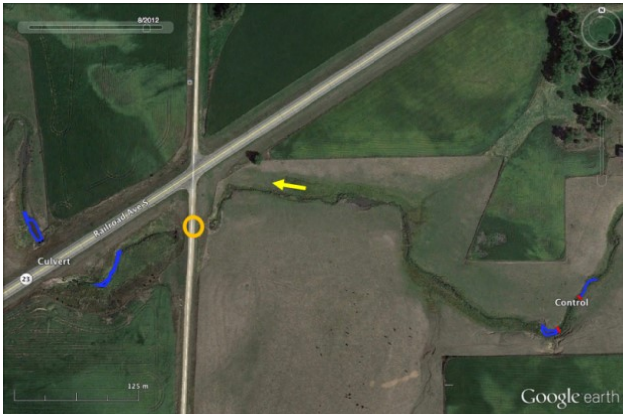
Figure 2.7 Satellite image (Google Earth) of culvert 8884 and corresponding control area (imagery taken 8/2012). Image shows a second culvert (orange circle) in between the experimental culvert and control reach. Blue delineates fish sampling areas, and red lines show the control stream reach. Stream direction is shown by the yellow arrow.
