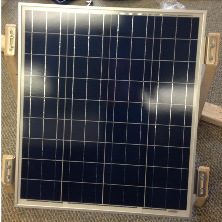
Figure 3-30 Solar Panel, 70 Watt
