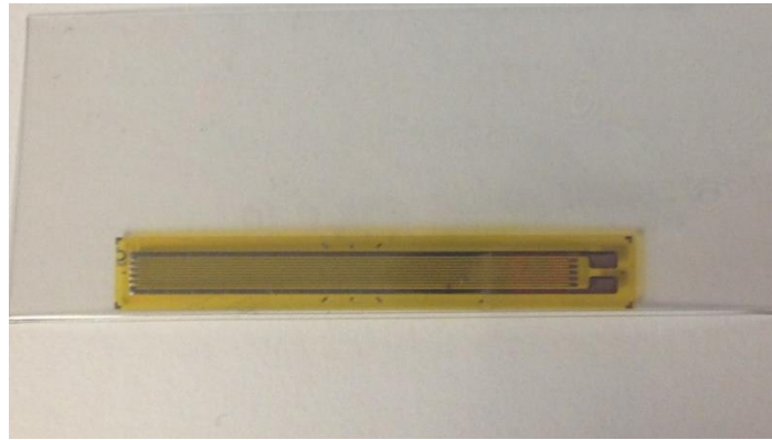
Figure 3-14 Concrete Strain Gage
