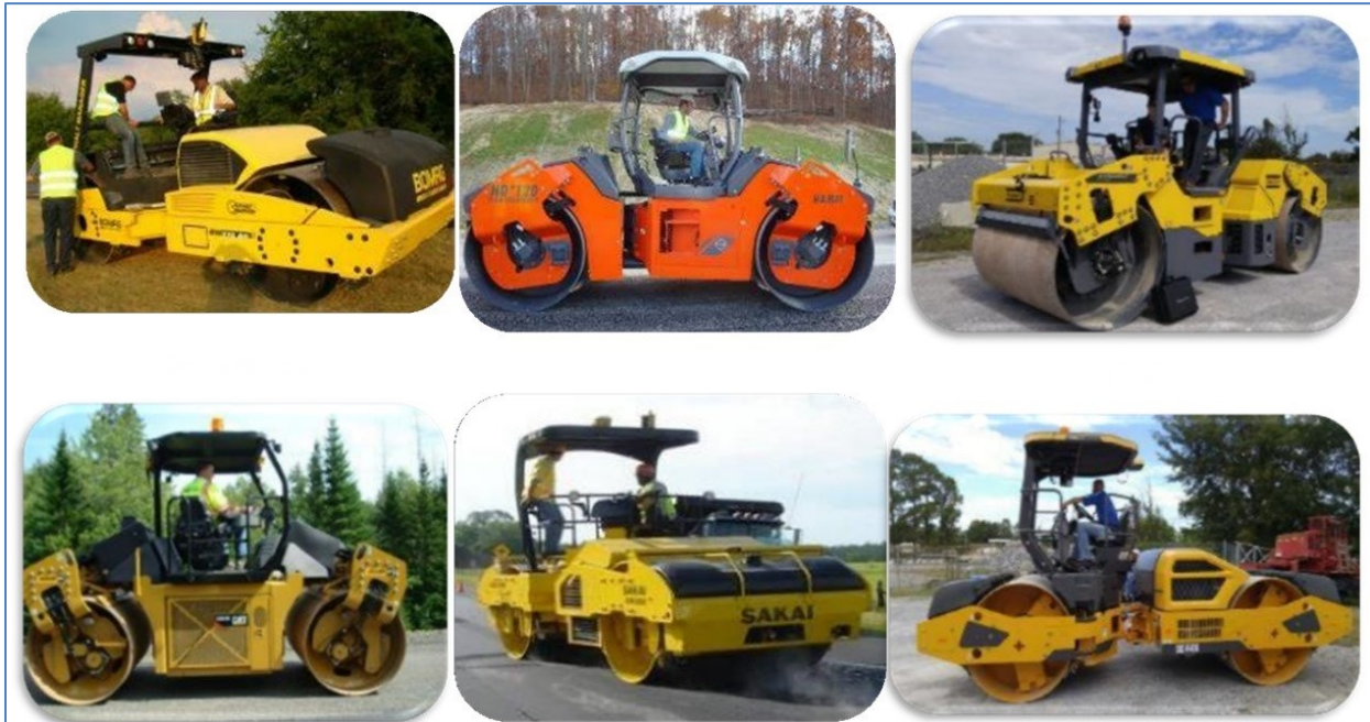
Figure 3. Examples of OEM Double-Drum IC Rollers.
