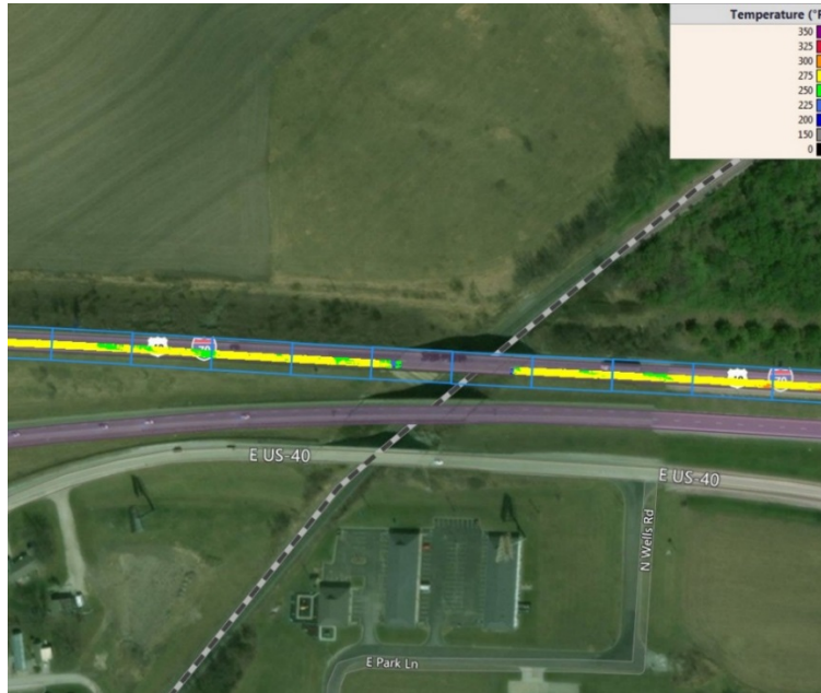
Figure 21: Example of a Veta Sublot screen for IR data analysis (J3I3042, RT70).
