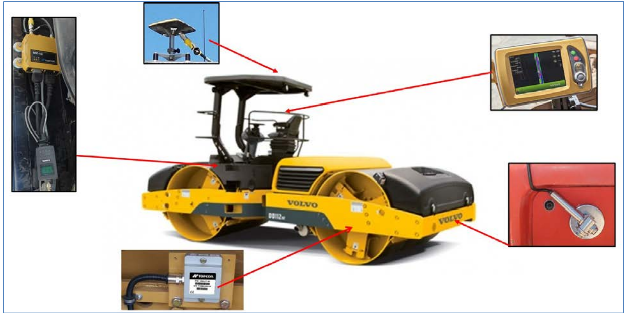
Figure 4. An Example of IC Retrofit Systems.
