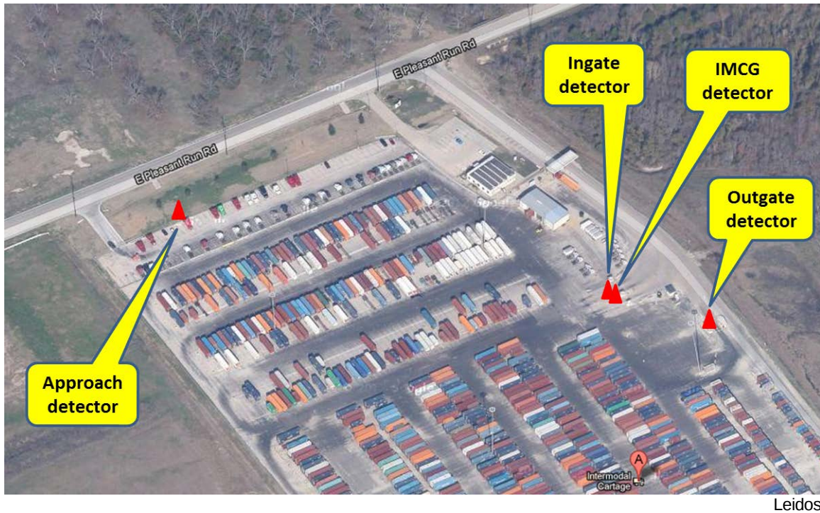
Figure 4. Bluetooth/Wi-Fi Reader Location at IMCG-Wilmer
