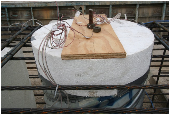
(e) PSV-28A Polystyrene Plug Secured with All-Thread Rod
