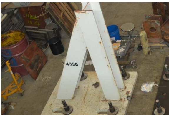
(a) Bottom Horizontal Actuator Reaction Frame
