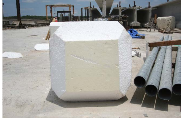
(b) PSV-28B Interior Void Polystyrene Forming Block (span) - Side
