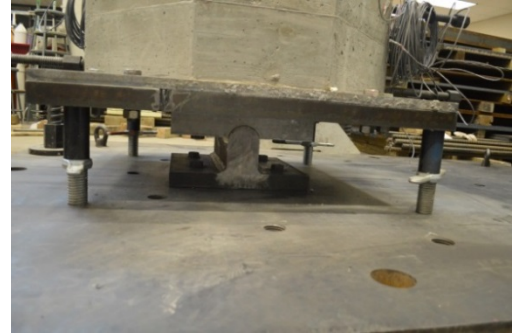
Figure 4.58. Rocker Foundation (Pegs Removed prior to Testing).
