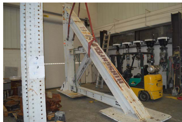
(b) Top Horizontal Actuator Reaction Frame
