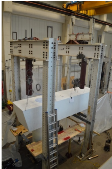
(a) Vertical Reaction Towers
