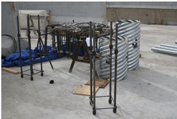
(a) All-Thread Actuator Load Assembly (Typ. for both Phase 1 and Phase 2)
