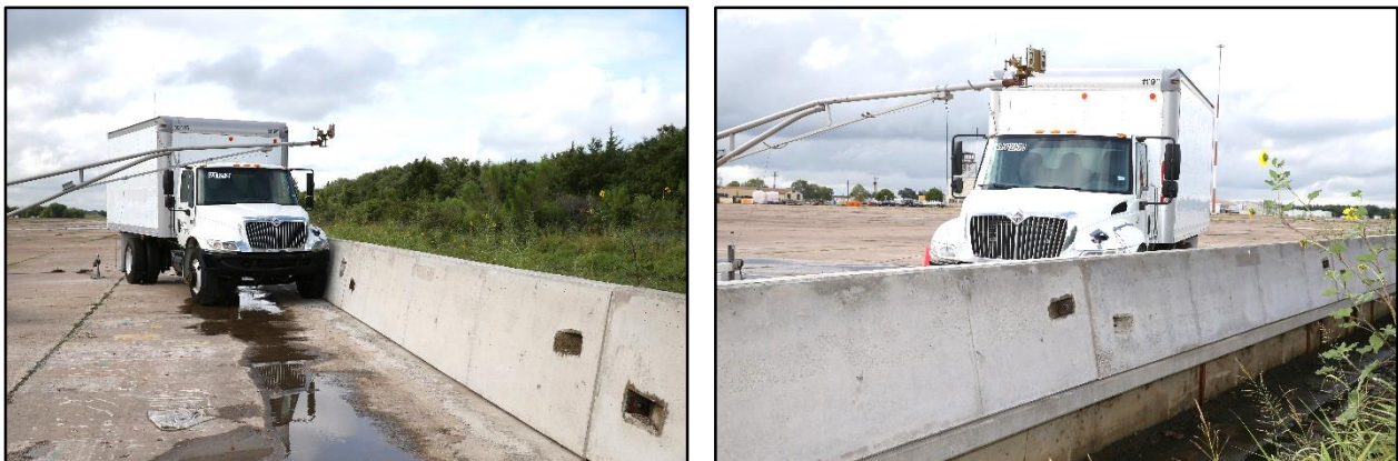
Figure 6.1. Restrained Barrier/Test Vehicle Geometrics for Test No. 490027-2-1.
