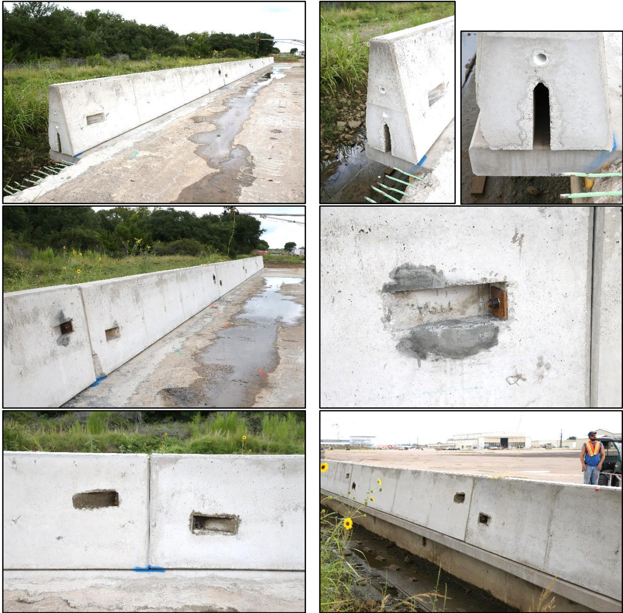
Figure 3.9. Restrained Safety-Shape Concrete Barrier on Concrete Bridge Deck prior to Testing.
