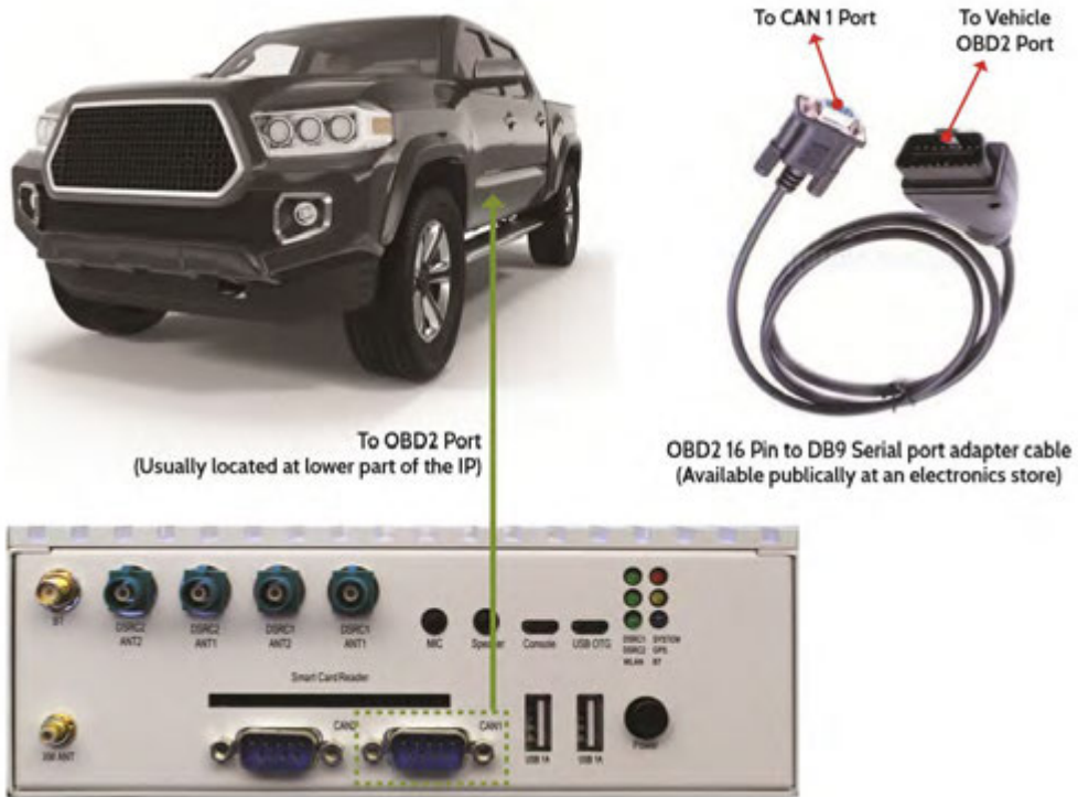
Figure 4-6. Lear Locomate Roadstar Premium CAN Bus Installation
