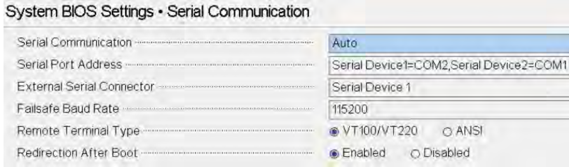
Figure 7-8. Default BIOS Serial Communication Settings
