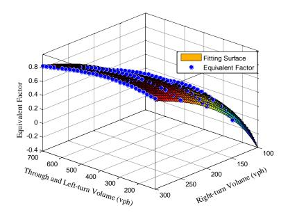
Figure 12 Regression Model Example for Configuration 4: main street volume =400 vph; VR=1:4
