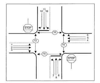
Figure 2 Movement Numbers for Right-turn Volume Adjustment
