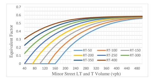
Figure 6 Equivalent Factor Graph for One Study Situation: main street volume= 500 vph; VR= 1:1
