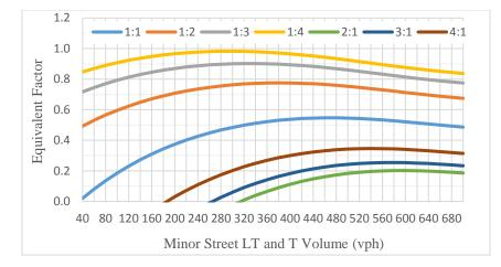
Figure 8 Equivalent factor Graph for Mainline Volume 500 vph
