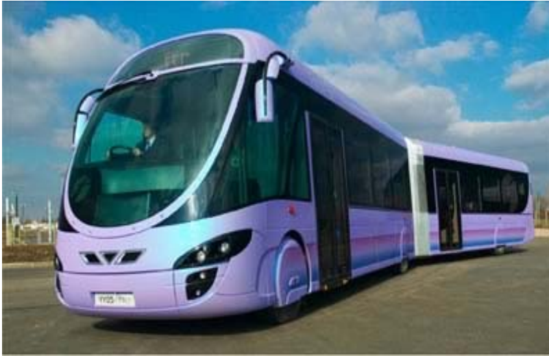
Figure 4-1: An illustration of one of the 50 new BRT vehicles to be added to the MAX fleet. This vehicle is being manufactured by the Wright Group of Northern Ireland. It will resemble the CIVIS but will not have optical guidance.
