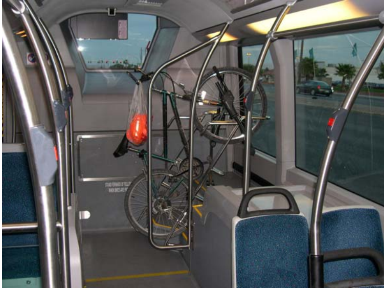
Figure 2-9: Onboard Bike Rack
