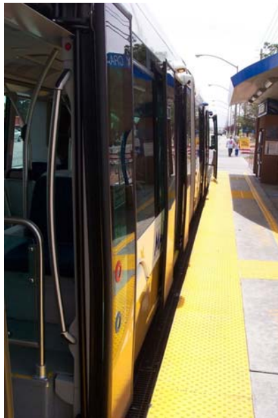
Figure 2-8b: MAX bus position at station using manual docking
