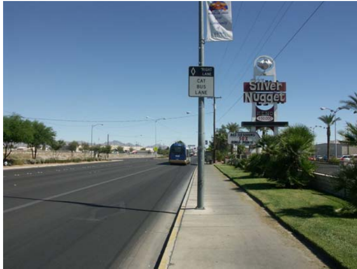
Figure 2-2: More than half of MAX's 7.5 mile route is an exclusive curbside bus lane
